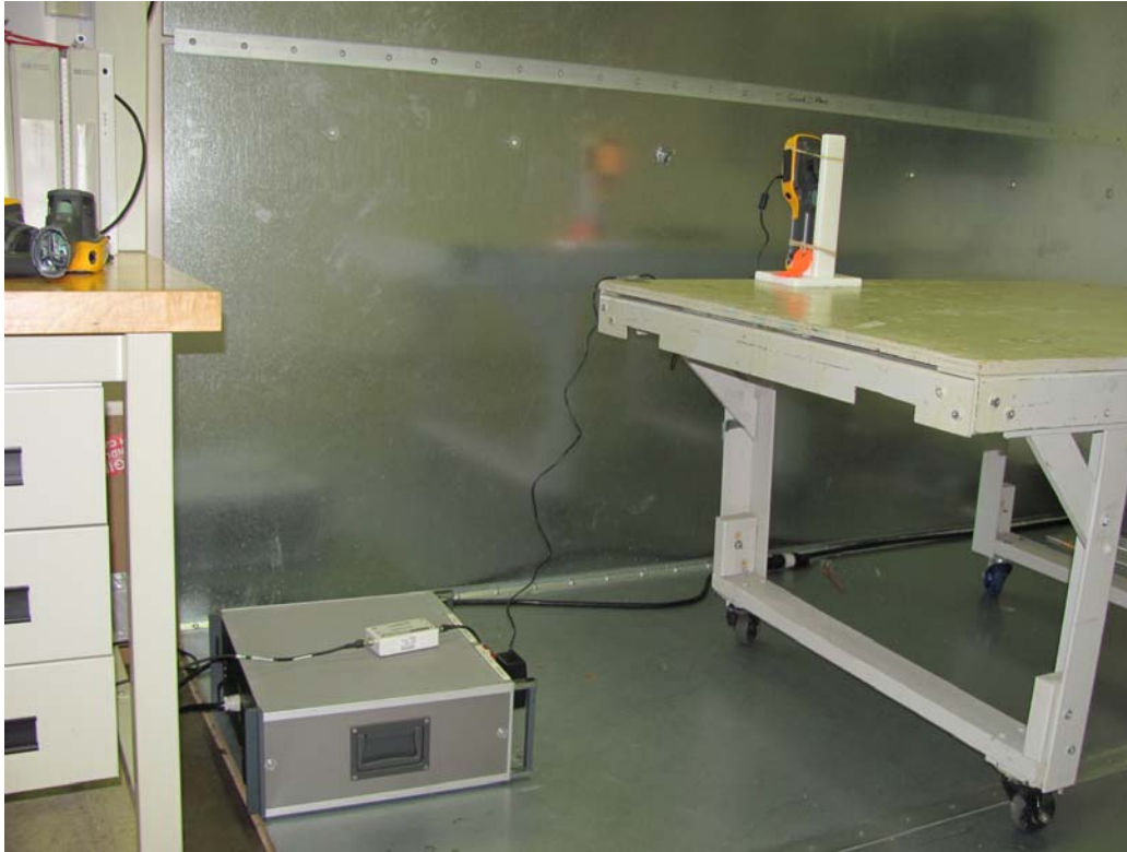
Figure 7: Conducted Emissions on AC Mains
