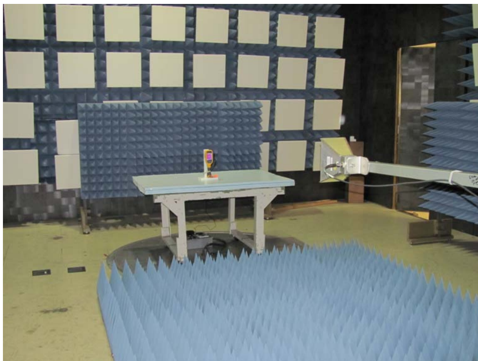
Figure 2: Radiated Emissions at 3m – 1 GHz to 18 GHz.
