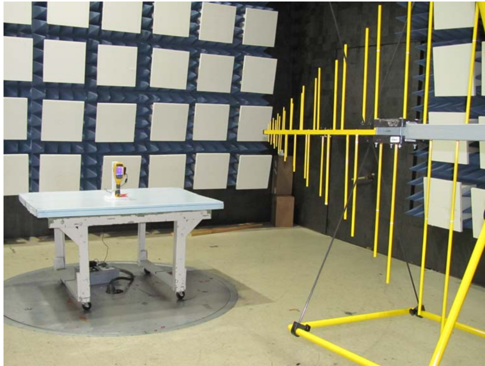
Figure 1: Radiated Emissions – 30 MHz to 1000 MHz.
