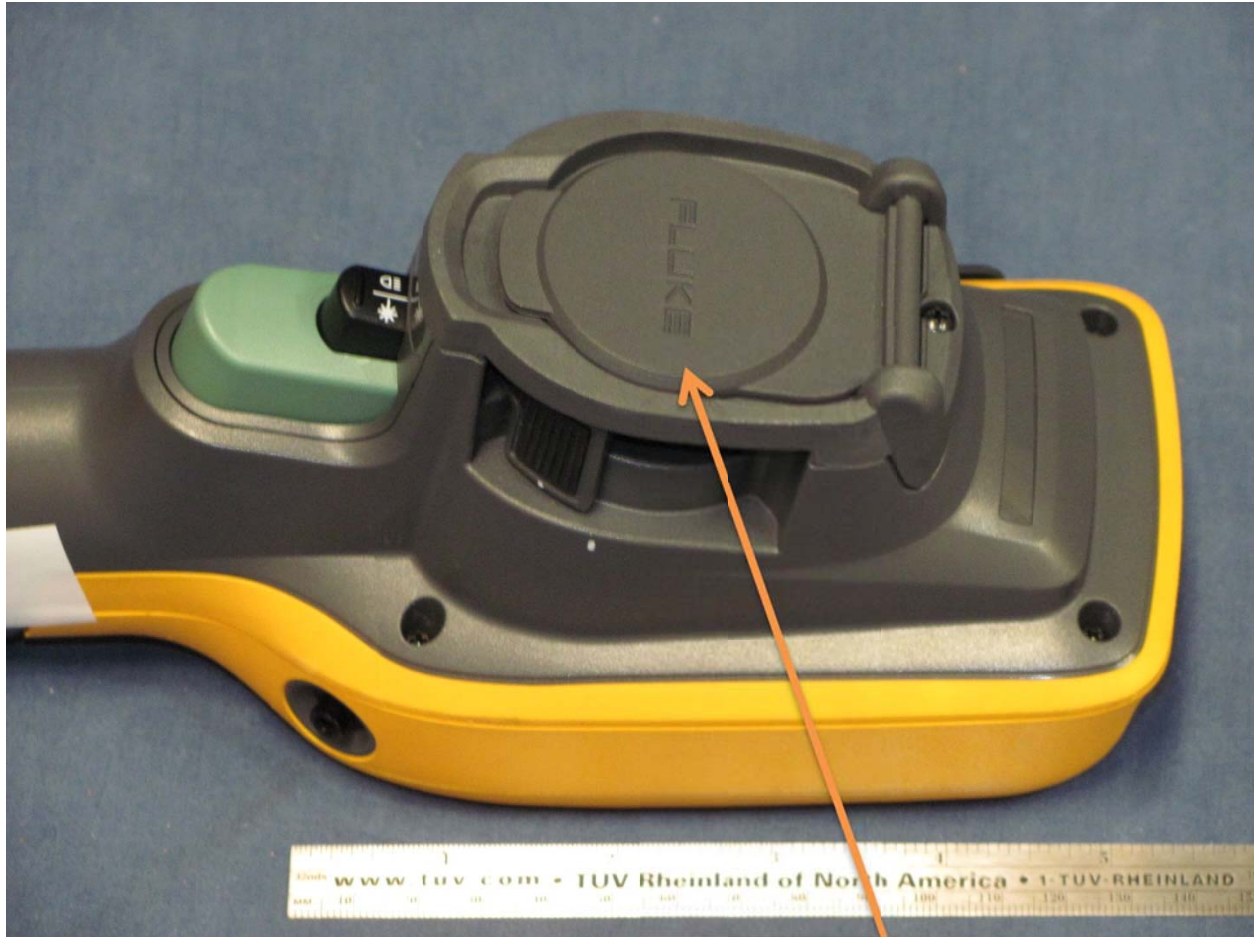
Rear View of EUT with imager lid closed. The Label will be placed on this lid See Label graphic.
