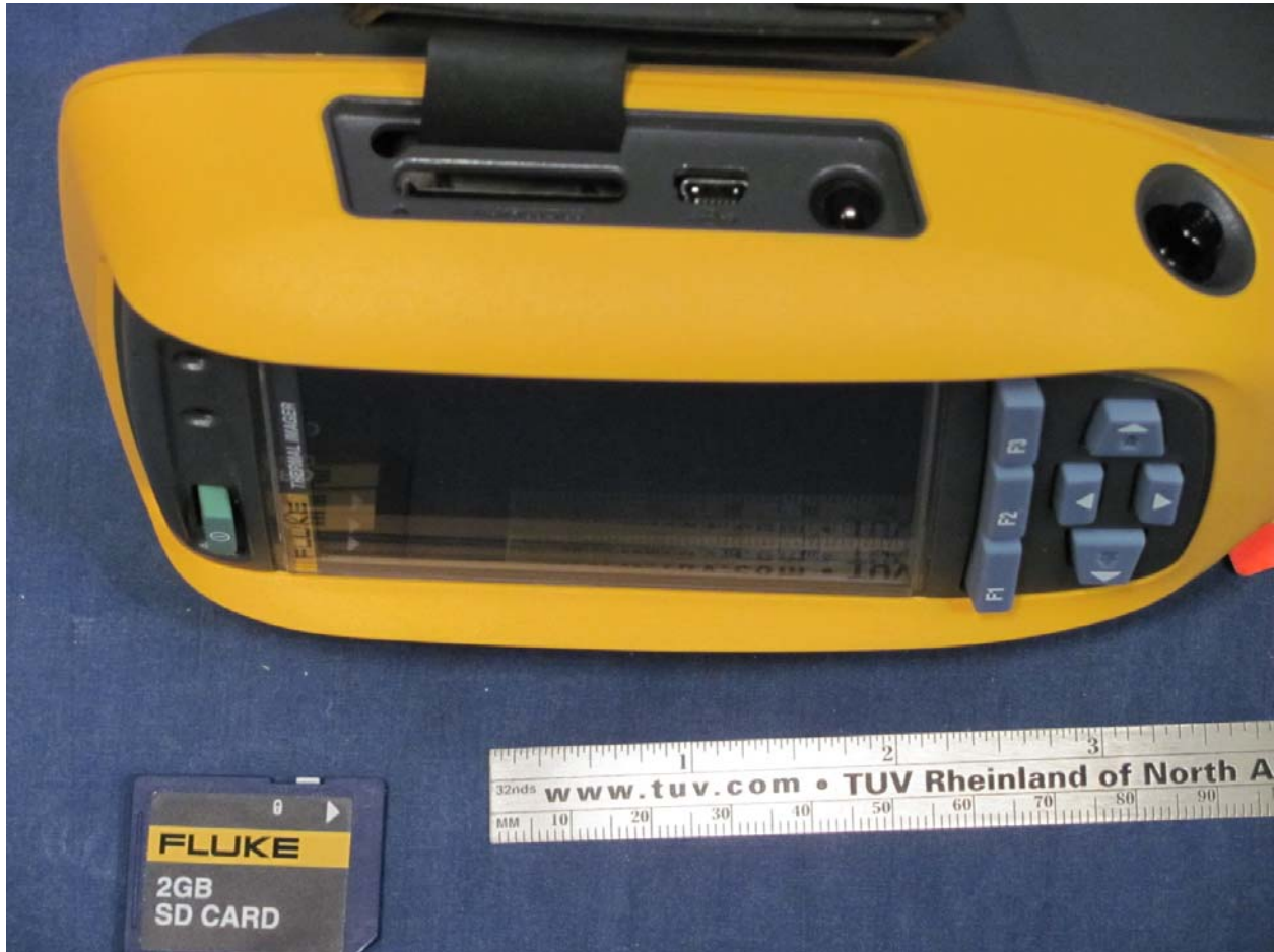
Figure 2: Edge view of test sample showing the SD card slot, USB slot and Power/charger connector.
