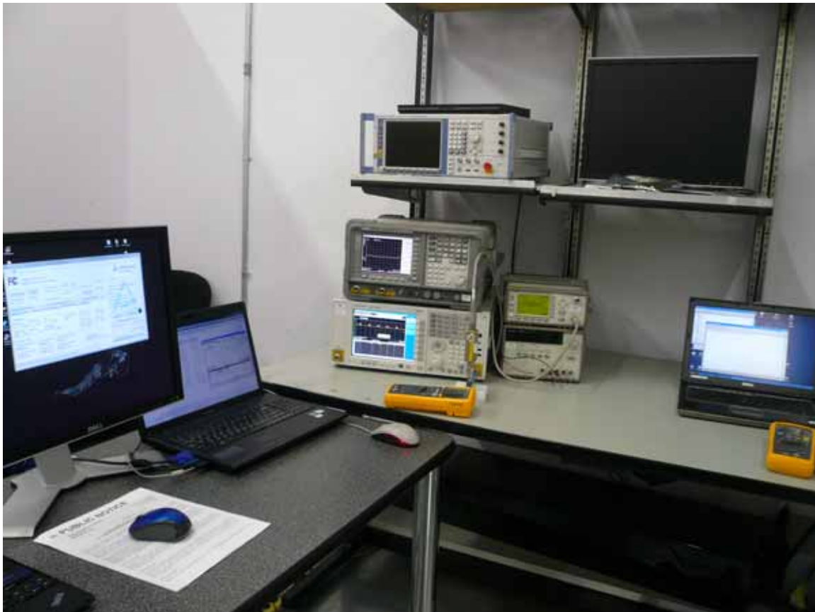
Figure 7: RF Conducted Test Setup
