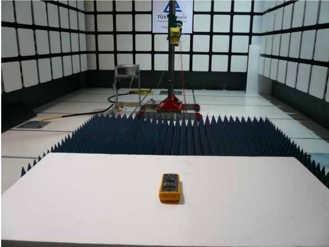
Figure 3: Test Setup for 1GHz to 18GHz (Front View)
