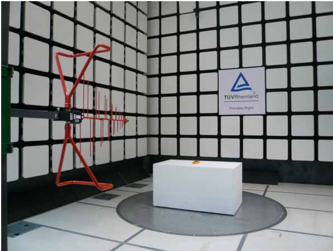
Figure 2: Test Setup for 30 MHz to 1000MHz (Rear View)
