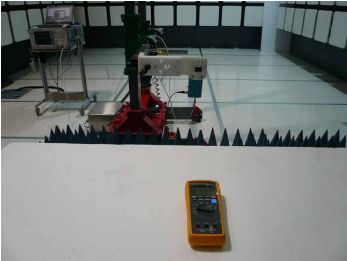
Figure 5: Test Setup for 18 GHz to 26GHz (Front View)
