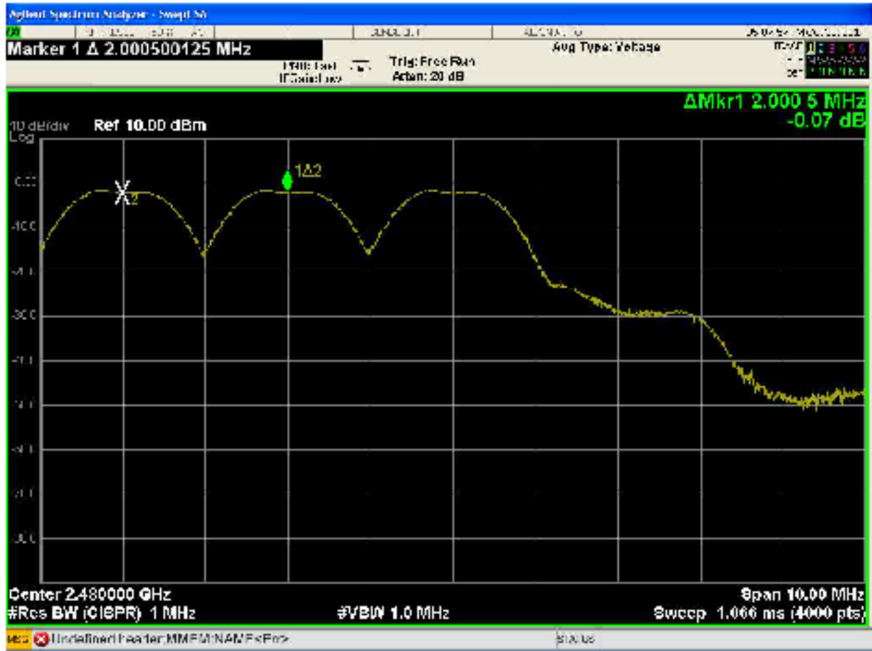
Figure 13: Channel Separation at 2480MHz
