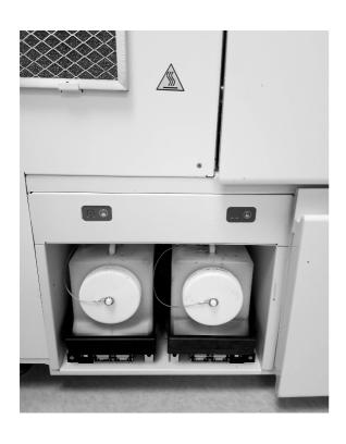
The VENTANA HE 600 system can collect liquid waste in waste containers or direct the waste to the drain.
