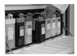
The automated fluidics module (AFM) stores and delivers the staining and cleaning reagents through a pressurized air and vacuum system. You can replace reagents by opening the AFM reagent access door.
