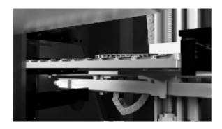
The transportation system moves slide trays between modules in the VENTANA HE 600 system.
