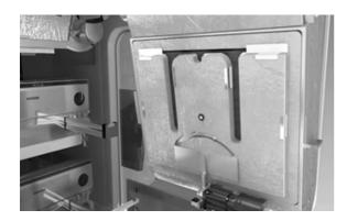
The slide dryer is a drying oven that ensures slides are dry and that paraffinized tissue sections are adhered to slides.
