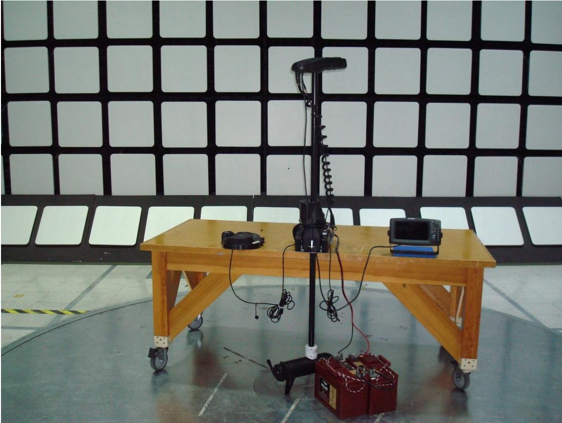
Figure 1 – Radiated Emissions Test Setup
