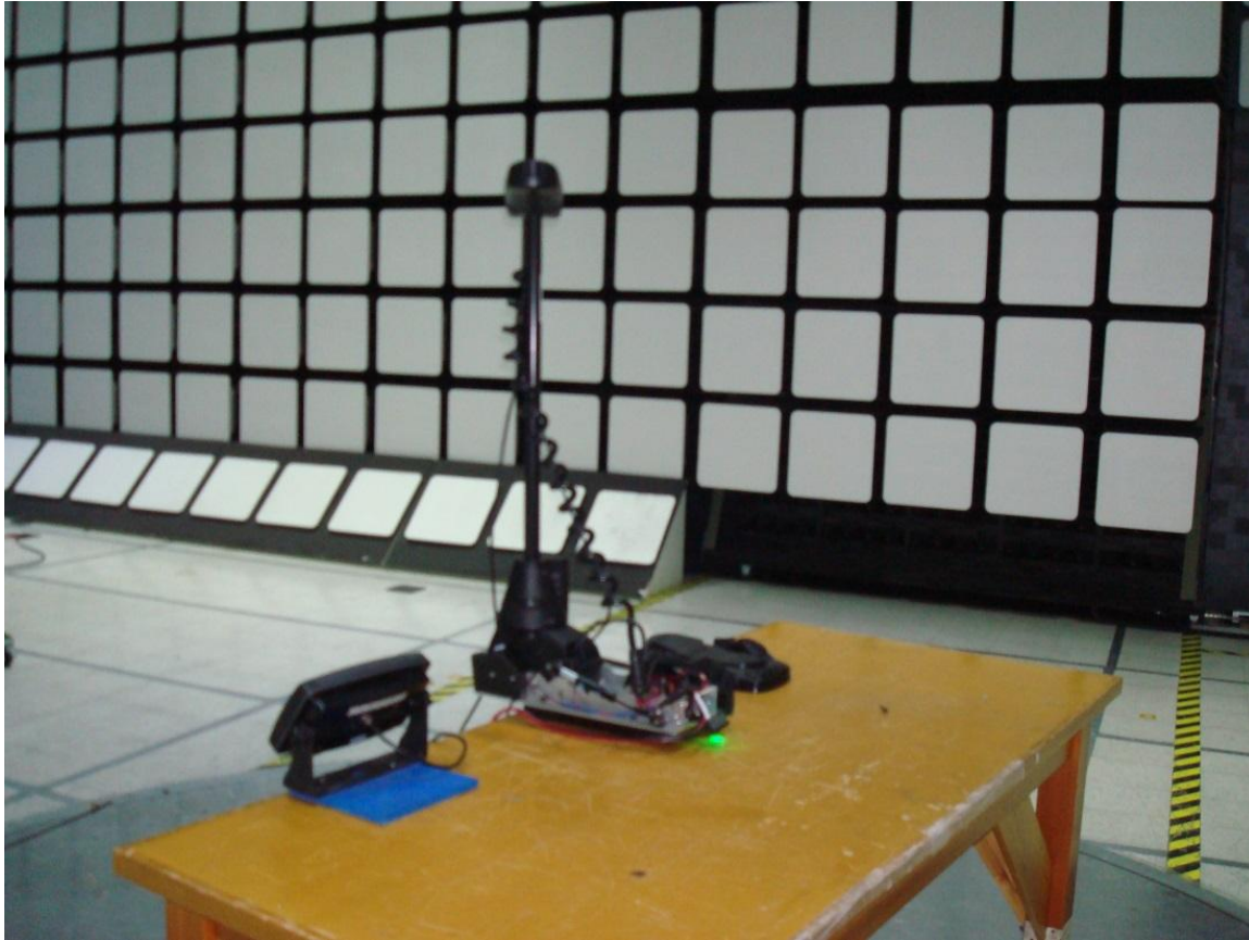
Figure 2 - Radiated Emissions Test Setup
