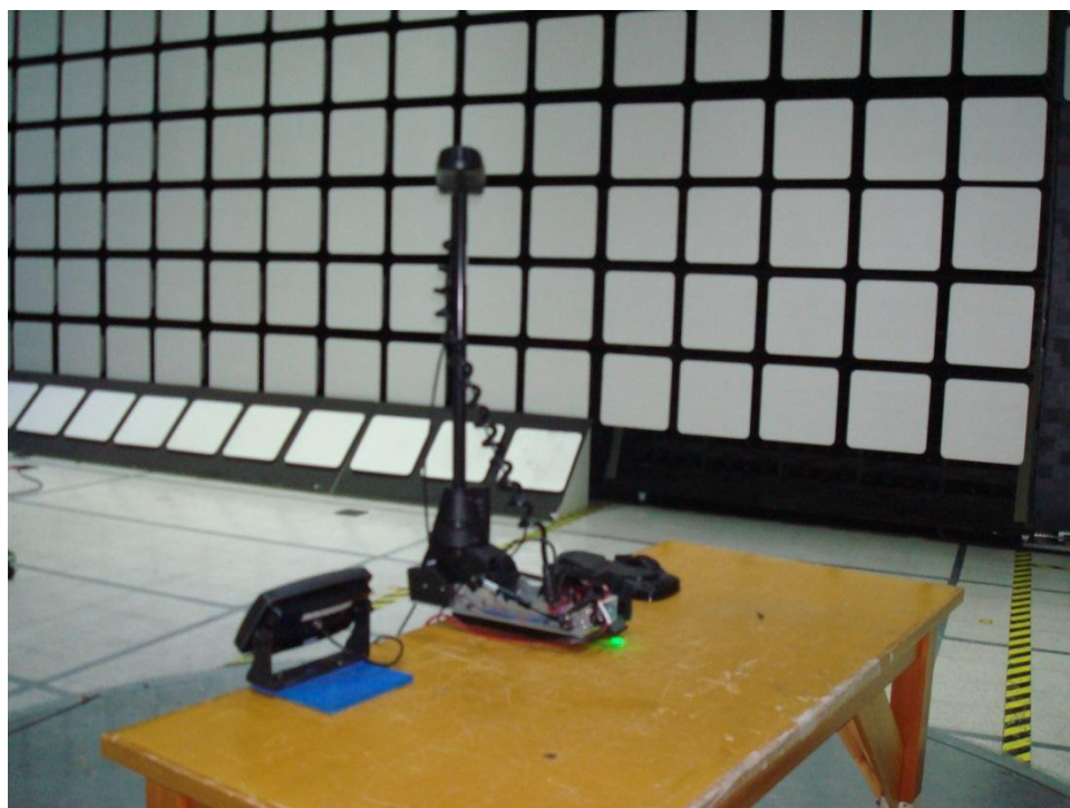
Figure 21 - Radiated Emissions Test Setup
