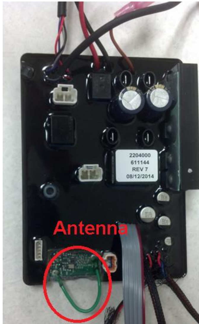
Figure 10 - Main Board with Potting. Antenna shown for 900 MHz band radio
