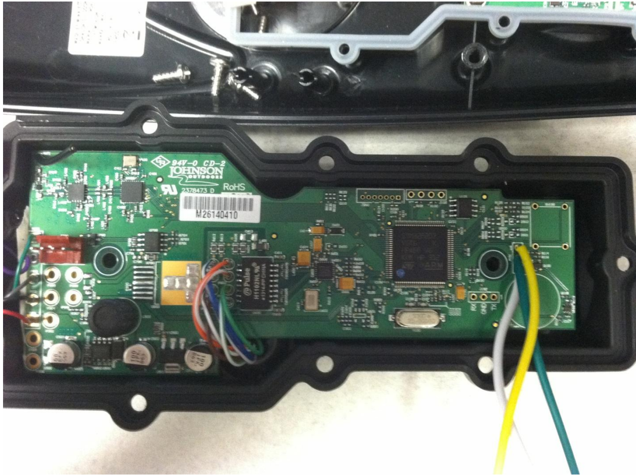
Figure 16 - iPilot Link circuit board (antenna shown in top left)
