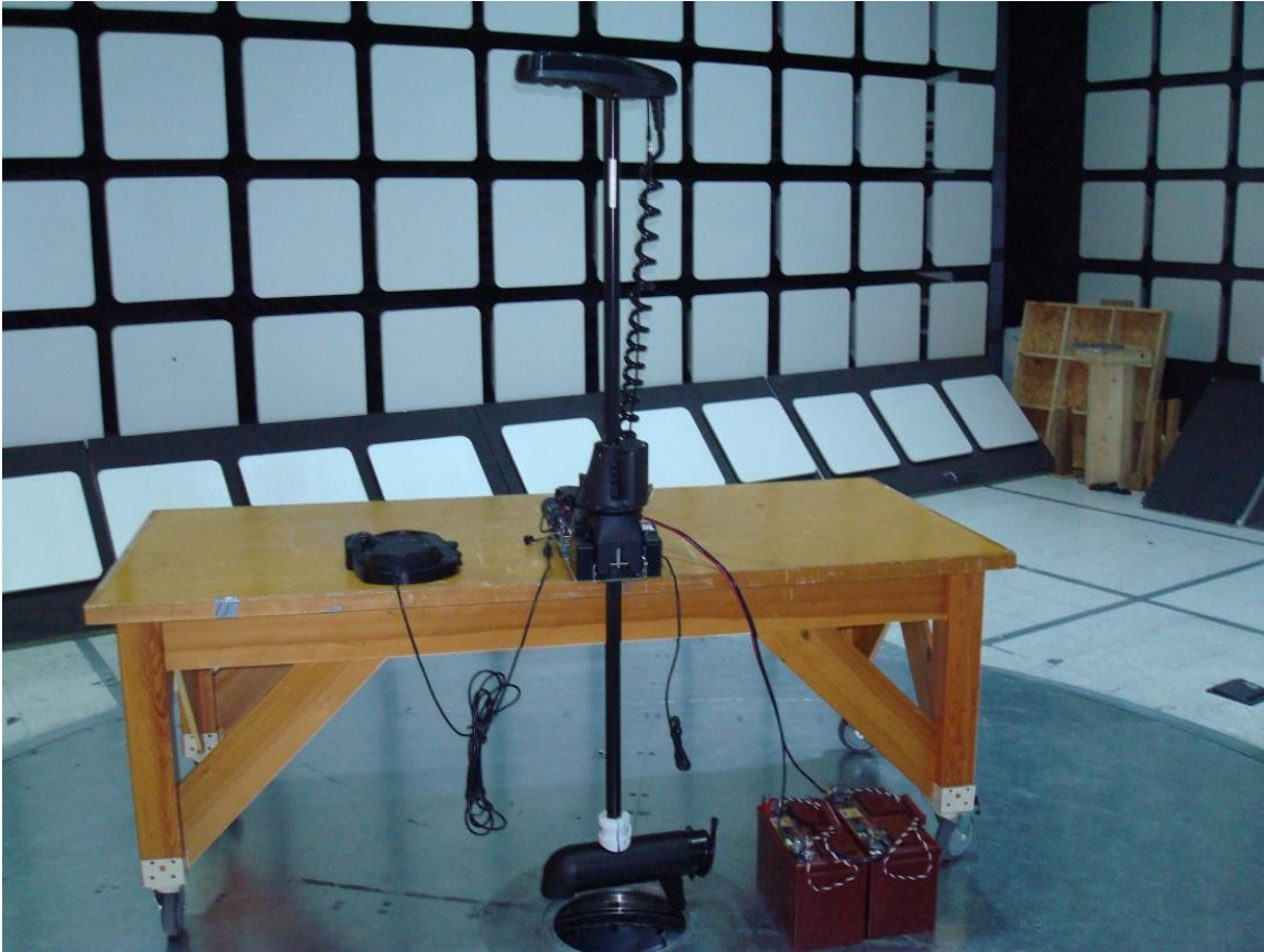
Figure 1 – Radiated Emissions Test Setup
