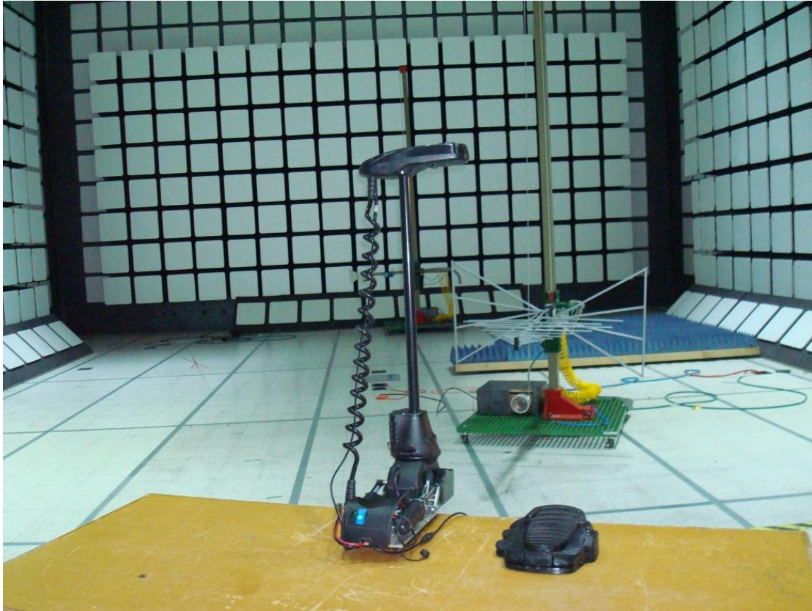
Figure 2 - Radiated Emissions Test Setup
