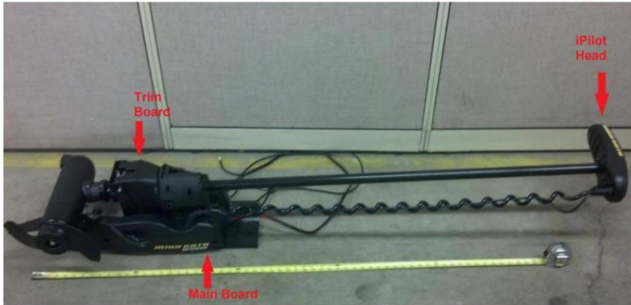
Figure 1 - Location of each circuit board assembly and radio
