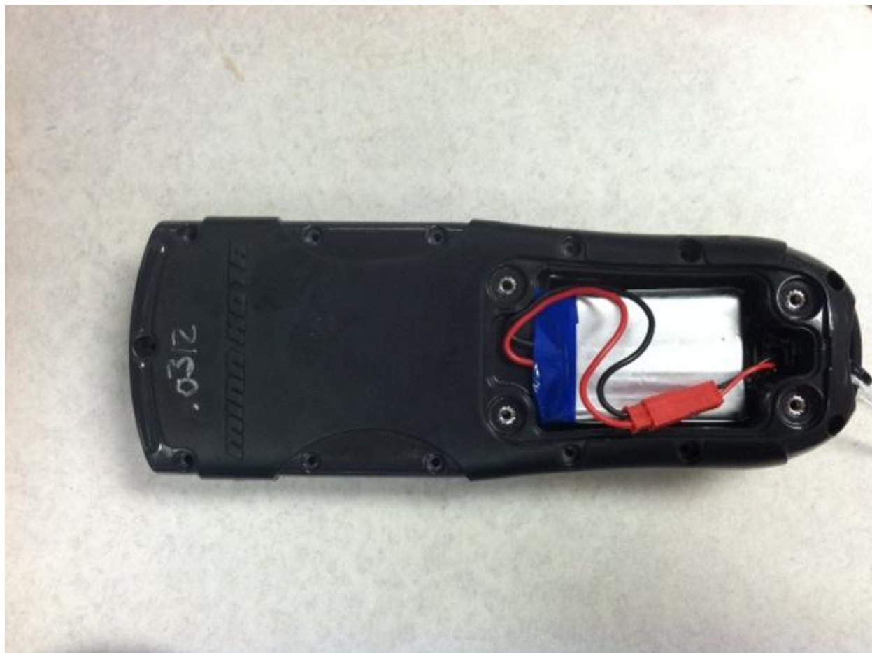
Figure 5 - Internal Photos, , Battery Compartment
