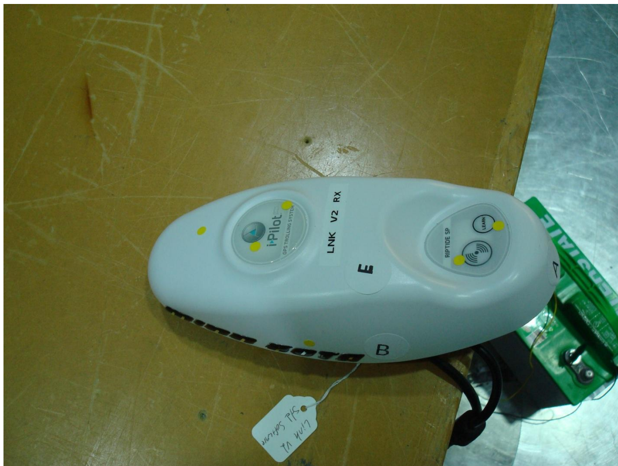
Figure 2 - i-Pilot Motor Controller Test Setup, Radiated Emissions
