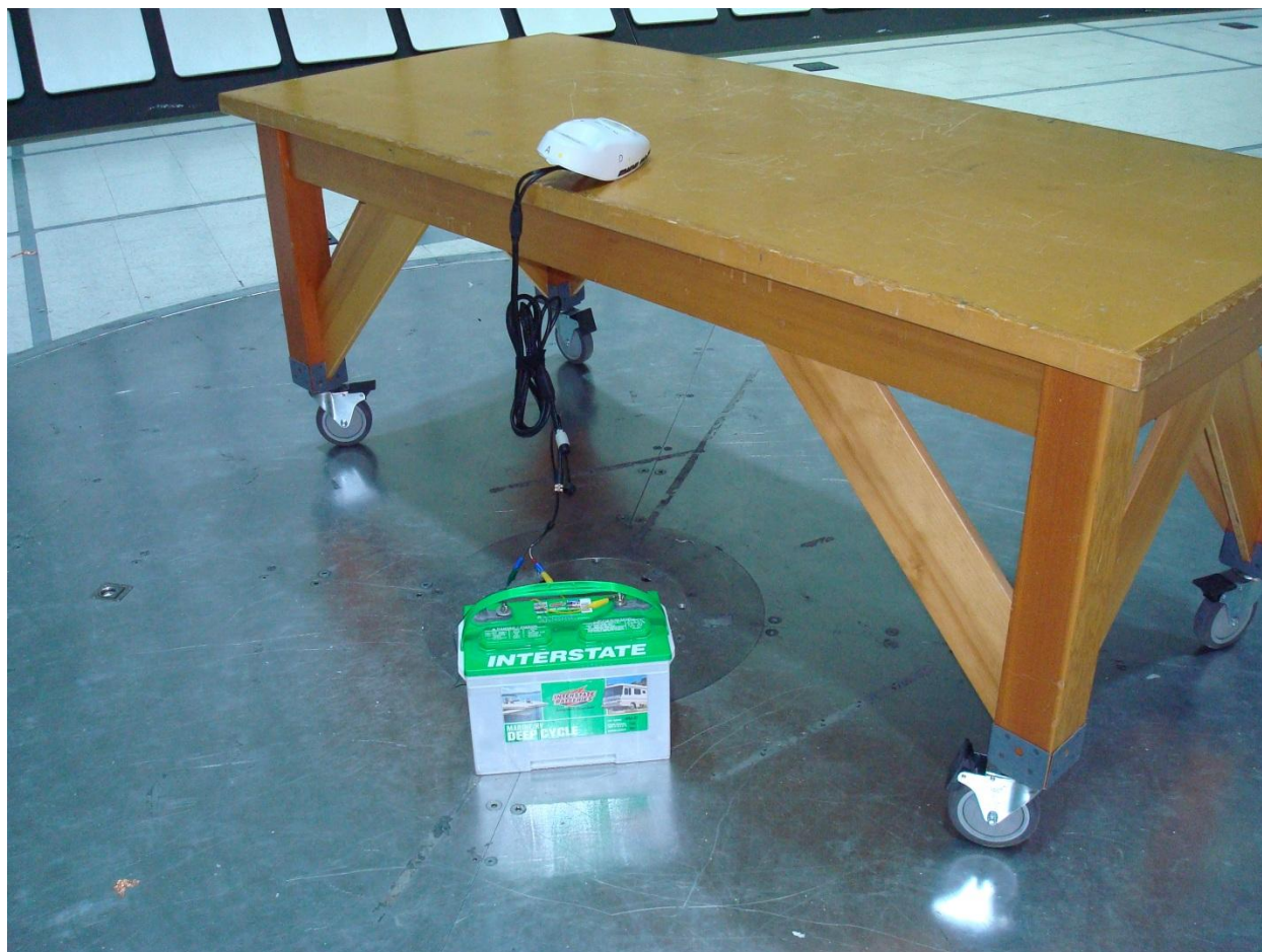
Figure 1 - i-Pilot Motor Controller Test Setup, Radiated Emissions
