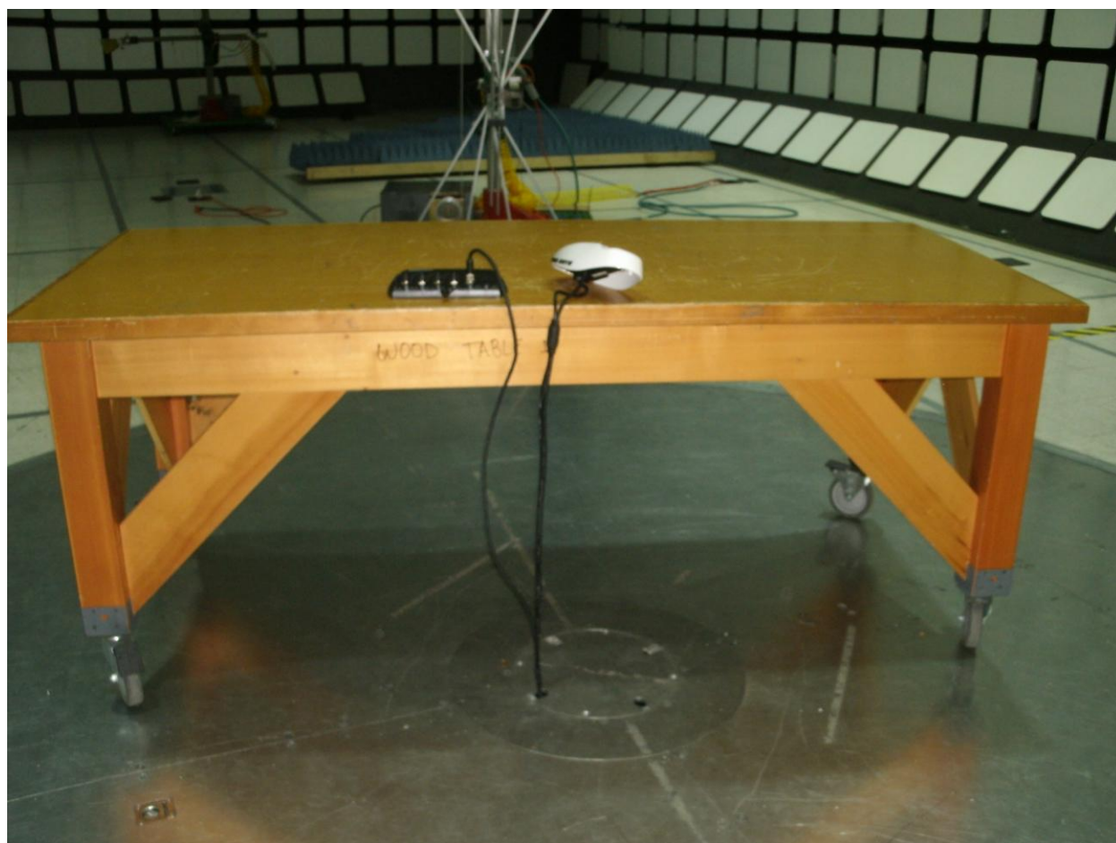
Figure 2 - EUT Test Setup with Modem Interface
