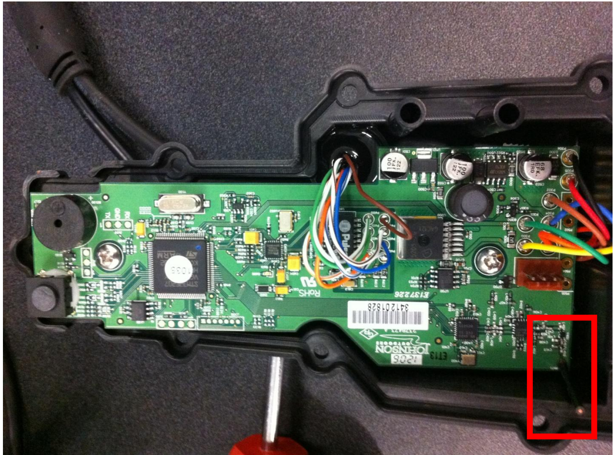
Figure 6 - Transmitter Board, antenna in red box, more detail in Figure 13
