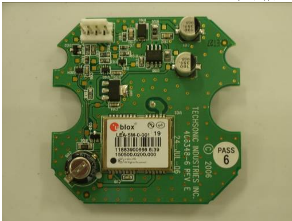
Figure 3 - i-Pilot Controller Internal, Daughter Board 1, Top
