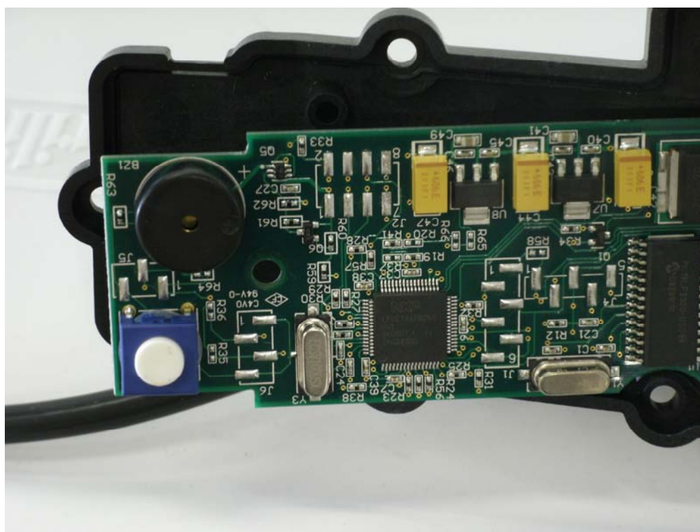
Figure 8 - i-Pilot Controller Internal, Main Board , Top, Left
