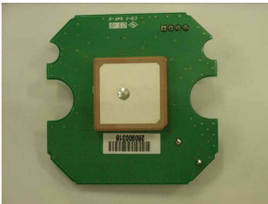
Figure 4 - i-Pilot Controller Internal, Daughter Board 1, Bottom
