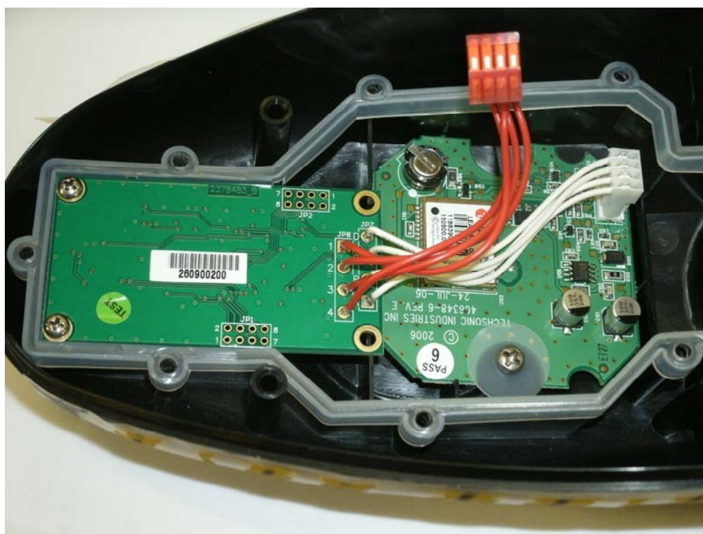
Figure 10 - i-Pilot Controller Internal, Daughter Boards Placement
