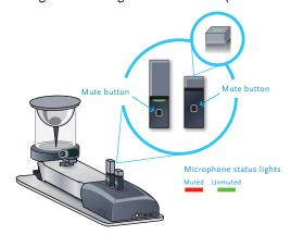
**Step 8** Attach the microphone to the speaker's clothing, within 6–12 inches of his or her mouth. Make sure microphone is attached securely with the microphone LED indicator pointed up toward mouth.
