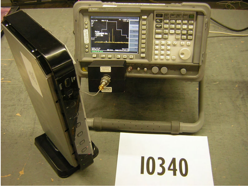
Antenna Port Conducted Measurements
