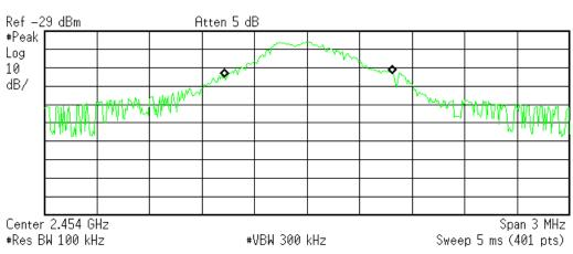
Occupied Bandwidth 960.7919 kHz Occ BW % Pwr 99.00 % x dB -26.00 dB
