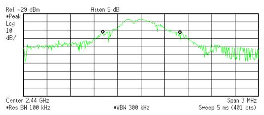
Occupied Bandwidth 982.3871 kHz Occ BW % Pwr 99.00 % x dB -26.00 dB
