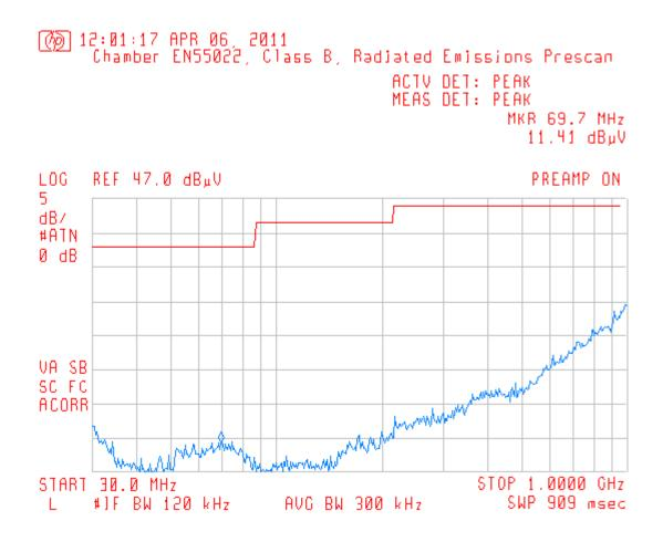
Prescan from Compact 3 Meter Chamber, no Measurable signals on 3 Meter OATS.
