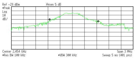
Occupied Bandwidth 1.1915 MHz Occ BW % Pwr 99.00 % x dB -26.00 dB
