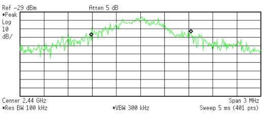
Occupied Bandwidth 1.2464 MHz Occ BW % Pwr 99.00 % x dB -26.00 dB
