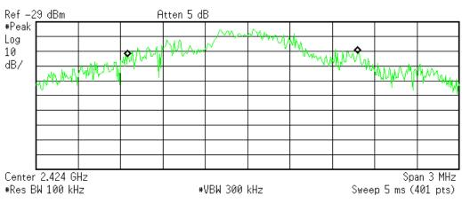
Occupied Bandwidth 1.6320 MHz Occ BW % Pwr 99.00 % x dB -26.00 dB
