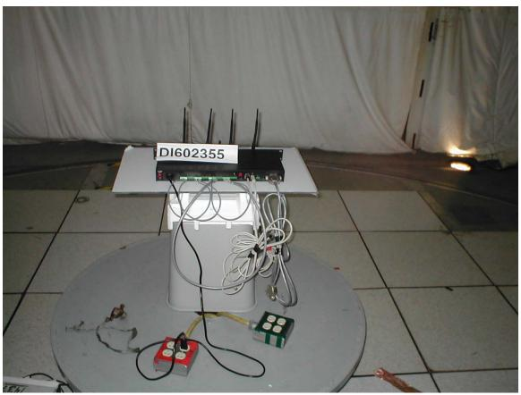
Test Set-up Conducted emissions – FCC Part 15.315
