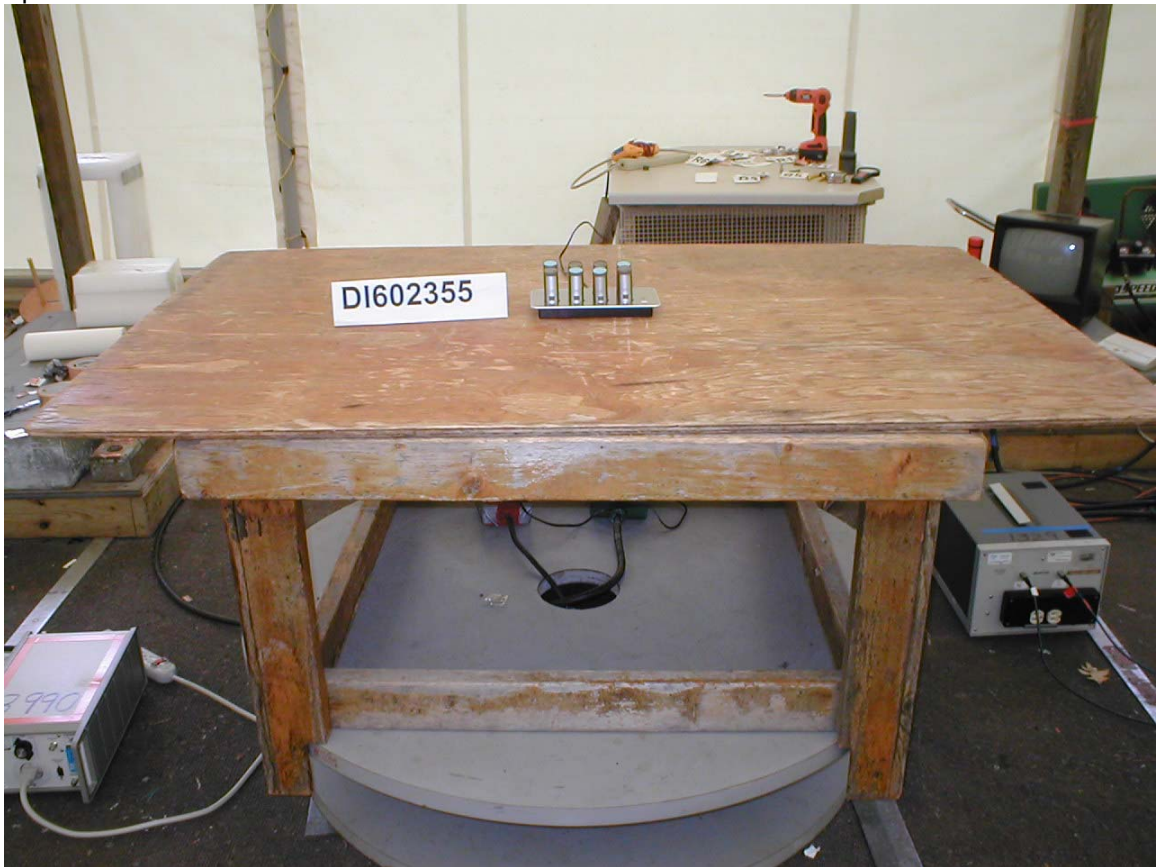
Test Set-up Photo Spurious emissions Part 15.309
