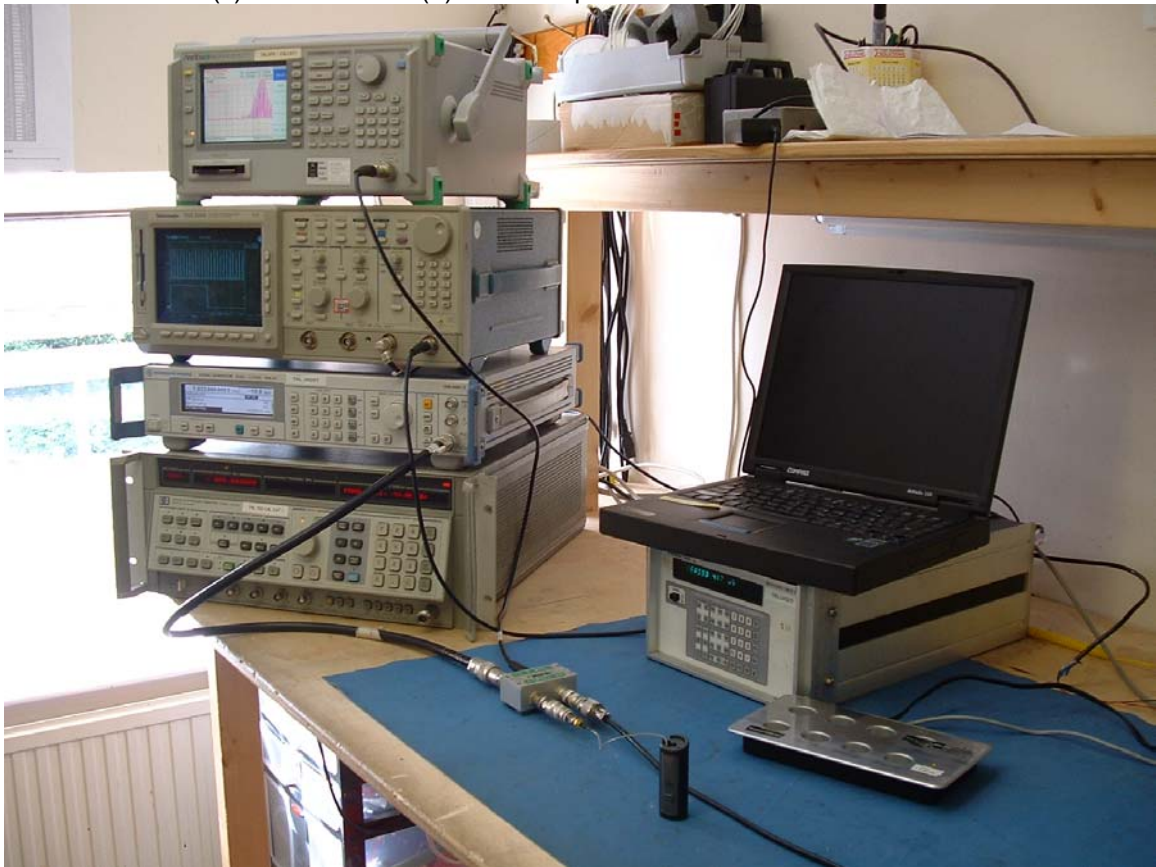
Test Set-up FCC Part 15.323 (c) & Part 15.323 (e) Test Setup
