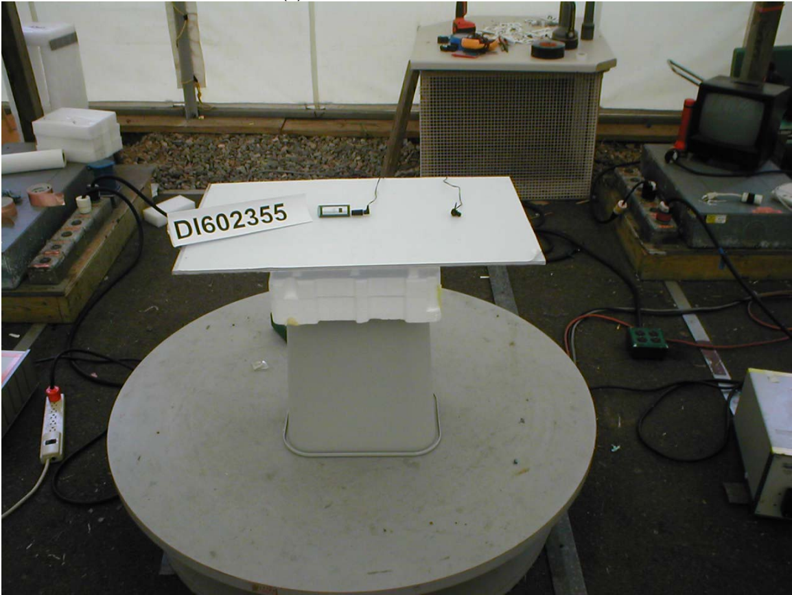
Test Set-up Radiated emissions – Part 15.319 (c)
