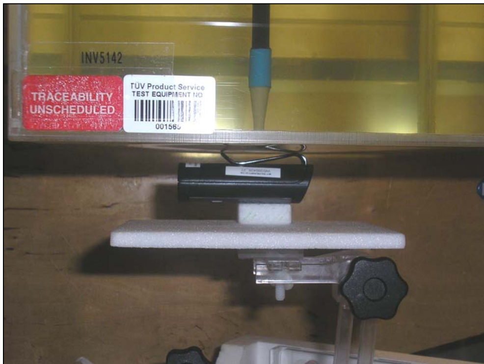
Figure 10: Positional Photograph of the Revolabs, Inc. C7490 Handset Rear Facing Phantom 0.0mm from the Phantom (SAR Body Test)
