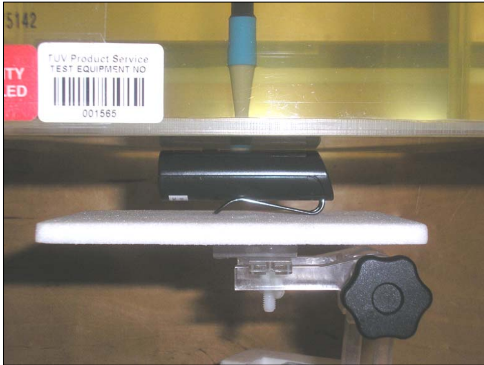
Figure 9: Positional Photograph of the Revolabs, Inc. C7490 Handset Front Facing Phantom 0.0mm from the Phantom (SAR Body Test)
