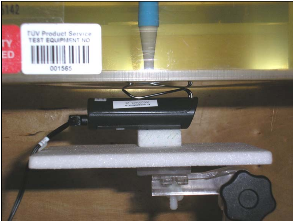
Figure 11: Positional Photograph of the Revolabs, Inc. C7490 Handset Front Facing Phantom 0.0mm from the Phantom with Ear Piece Accessory Attached (SAR Body Test)
