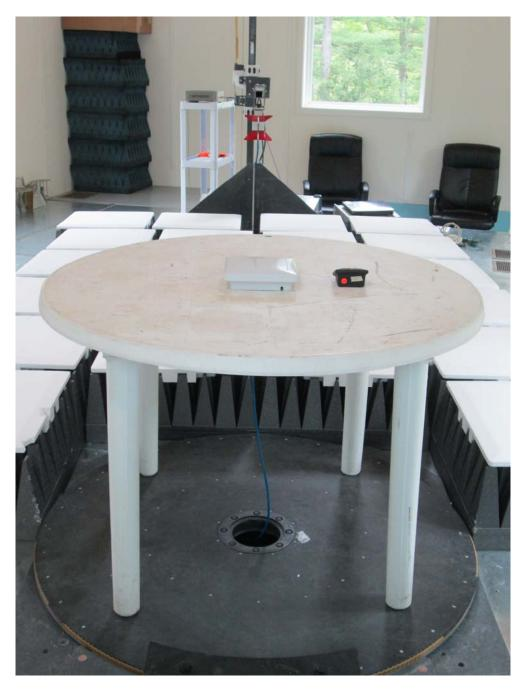
7. Test Images 7.5. Radiated Emissions – Front Above 1 GHz
