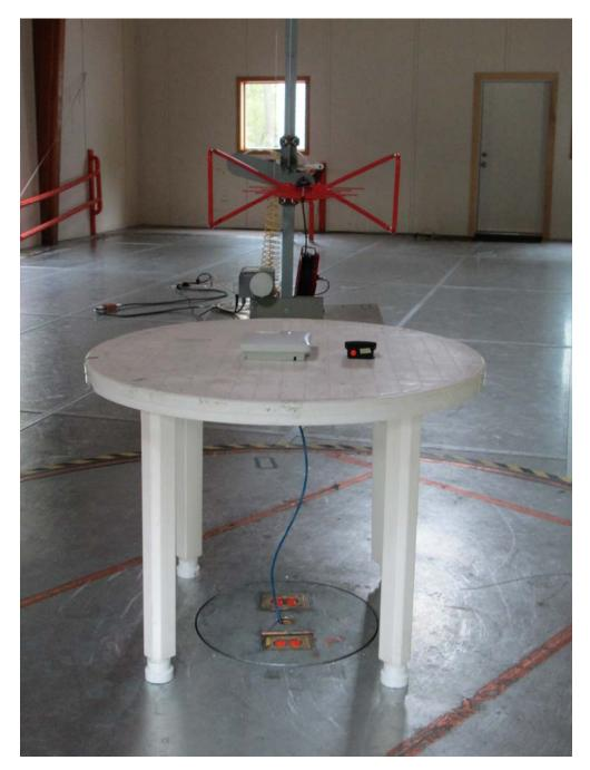
7. Test Images 7.3. Radiated Emissions – Rear 30 MHz to 1 GHz
