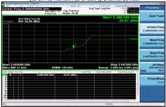
Band edge emission at antenna terminals -5MHz BW LTE-Band 41 (QPSK RB Number: 25 Offset: 0) Channel Highest
