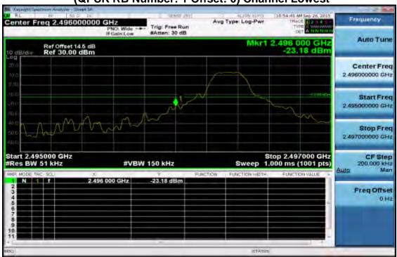
Band edge emission at antenna terminals - 5MHz BW LTE-Band 41 (QPSK RB Number: 1 Offset: 24) Channel Highest
