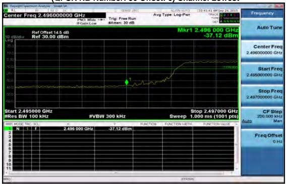
Band edge emission at antenna terminals - 10MHz BW LTE-Band 41 (QPSK RB Number: 50 Offset: 0) Channel Highest
