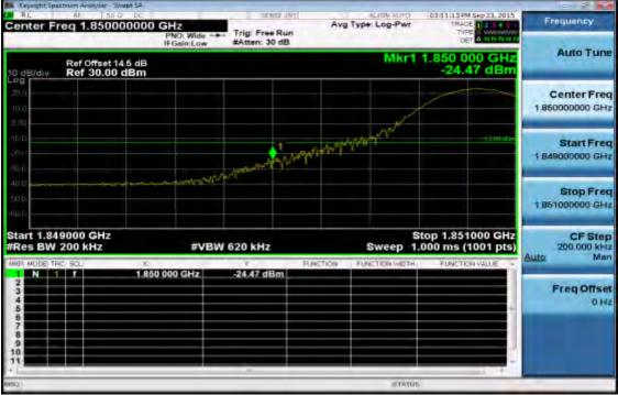
Band edge emission at antenna terminals –15MHz BW LTE-Band 2 (QPSK RB Number: 1 Offset: 74) Channel Highest
