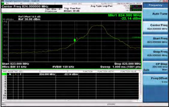
Band edge emission at antenna terminals –5MHz BW LTE-Band 5 (QPSK RB Number: 1 Offset: 24) Channel Highest
