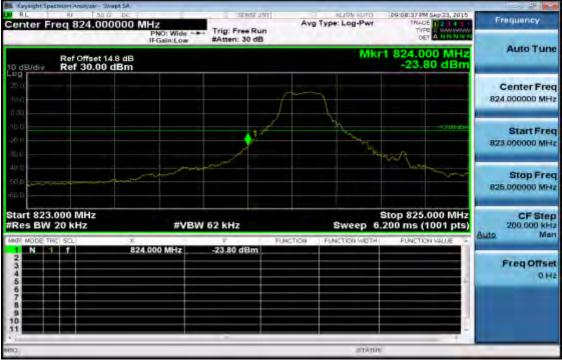
Band edge emission at antenna terminals -1.4MHz BW LTE-Band 5 (QPSK RB Number: 1 Offset: 5) Channel Highest
