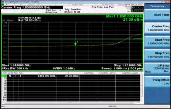
Band edge emission at antenna terminals -20MHz BW LTE-Band 2 (QPSK RB Number: 100 Offset: 0) Channel Highest
