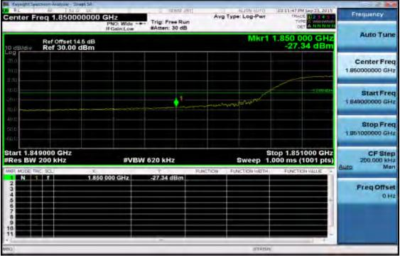
Band edge emission at antenna terminals –15MHz BW LTE-Band 2 (QPSK RB Number: 75 Offset: 0) Channel Highest
