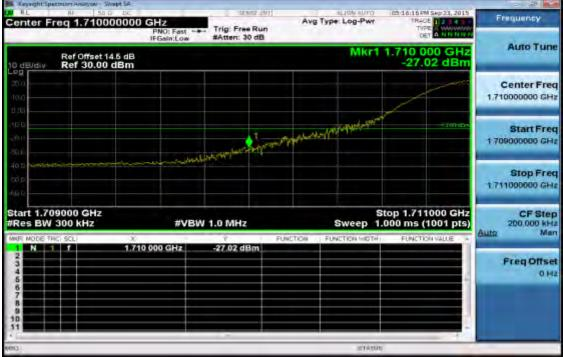
Band edge emission at antenna terminals -20MHz BW LTE-Band 4 (QPSK RB Number: 1 Offset: 99) Channel Highest
