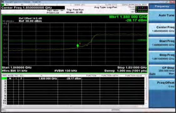
Band edge emission at antenna terminals –5MHz BW LTE-Band 2 (QPSK RB Number: 25 Offset: 0) Channel Highest
