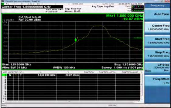
Band edge emission at antenna terminals –5MHz BW LTE-Band 2 (QPSK RB Number: 1 Offset: 24) Channel Highest
