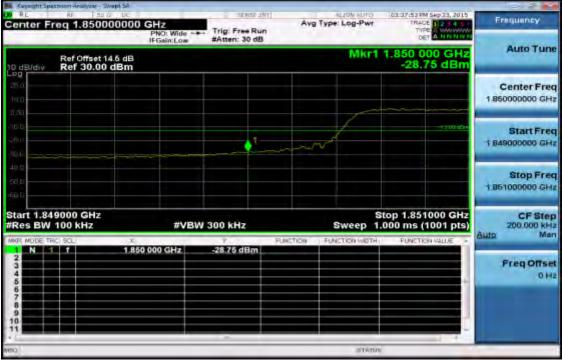
Band edge emission at antenna terminals -10MHz BW LTE-Band 2 (QPSK RB Number: 50 Offset: 0) Channel Highest
