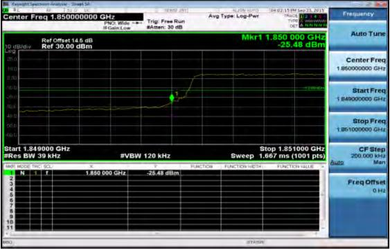
Band edge emission at antenna terminals –3MHz BW LTE-Band 2 (QPSK RB Number: 15 Offset: 0) Channel Highest
