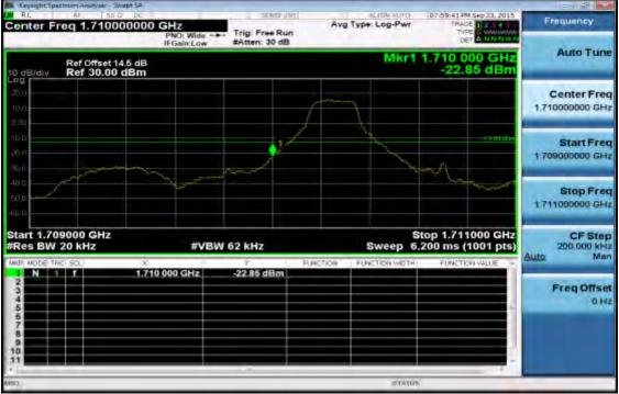
Band edge emission at antenna terminals -1.4MHz BW LTE-Band 4 (QPSK RB Number: 1 Offset: 5) Channel Highest
