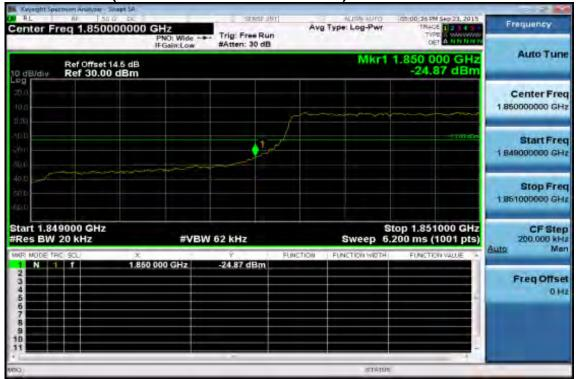
Band edge emission at antenna terminals -1.4MHz BW LTE-Band 2 (QPSK RB Number: 6 Offset: 0) Channel Highest
