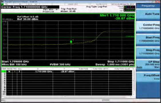
Band edge emission at antenna terminals -10MHz BW LTE-Band 4 (QPSK RB Number: 50 Offset: 0) Channel Highest
