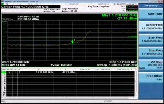
Band edge emission at antenna terminals –5MHz BW LTE-Band 4 (QPSK RB Number: 25 Offset: 0) Channel Highest
