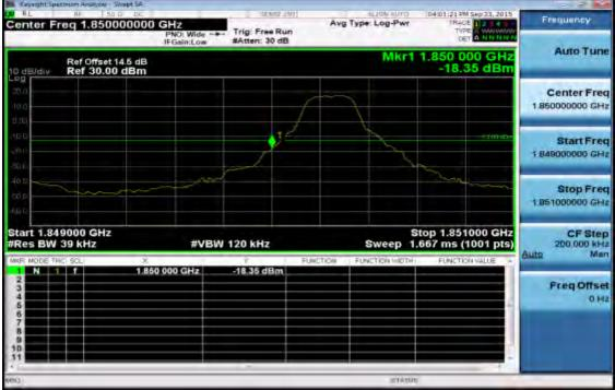
Band edge emission at antenna terminals –3MHz BW LTE-Band 2 (QPSK RB Number: 1 Offset: 14) Channel Highest
