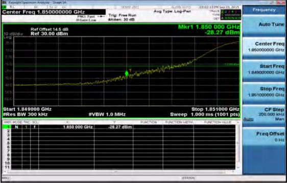
Band edge emission at antenna terminals –20MHz BW LTE-Band 2 (QPSK RB Number: 1 Offset: 99) Channel Highest
