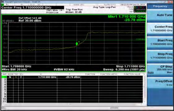
Band edge emission at antenna terminals -1.4MHz BW LTE-Band 4 (QPSK RB Number: 6 Offset: 0) Channel Highest
