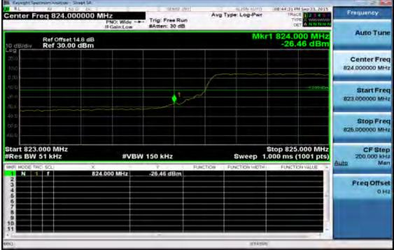
Band edge emission at antenna terminals –5MHz BW LTE-Band 5 (QPSK RB Number: 25 Offset: 0) Channel Highest
