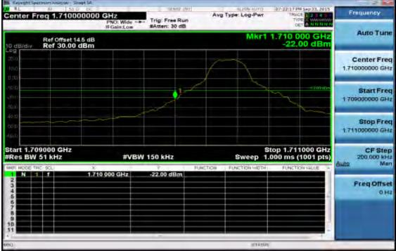
Band edge emission at antenna terminals –5MHz BW LTE-Band 4 (QPSK RB Number: 1 Offset: 24) Channel Highest
