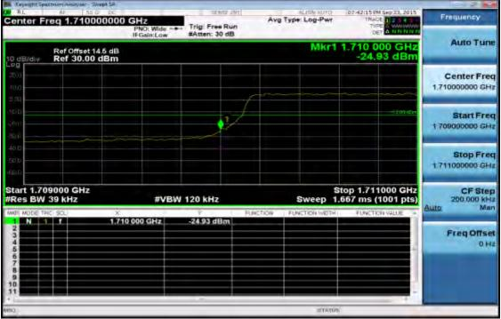
Band edge emission at antenna terminals –3MHz BW LTE-Band 4 (QPSK RB Number: 15 Offset: 0) Channel Highest
