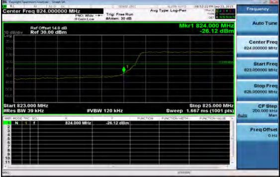
Band edge emission at antenna terminals –3MHz BW LTE-Band 5 (QPSK RB Number: 15 Offset: 0) Channel Highest
