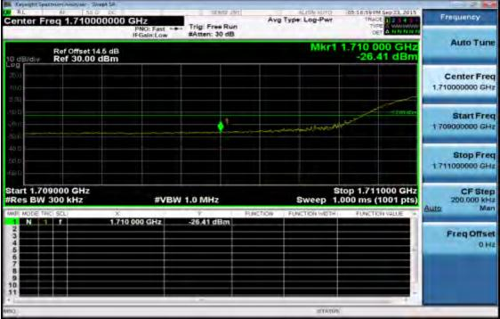
Band edge emission at antenna terminals -20MHz BW LTE-Band 4 (QPSK RB Number: 100 Offset: 0) Channel Highest
