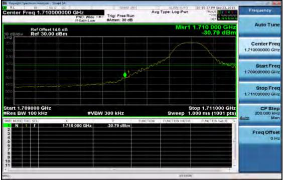
Band edge emission at antenna terminals -10MHz BW LTE-Band 4 (QPSK RB Number: 1 Offset: 49) Channel Highest
