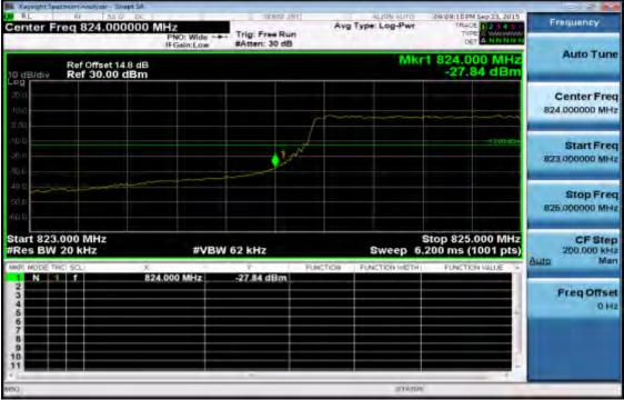
Band edge emission at antenna terminals -1.4MHz BW LTE-Band 5 (QPSK RB Number: 6 Offset: 0) Channel Highest
