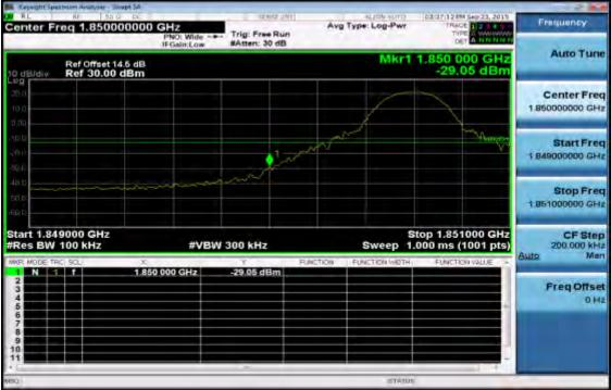
Band edge emission at antenna terminals –10MHz BW LTE-Band 2 (QPSK RB Number: 1 Offset: 49) Channel Highest
