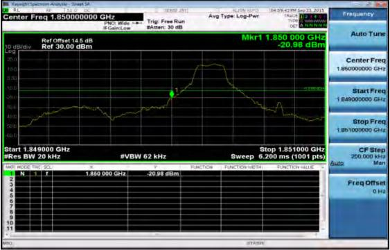
Band edge emission at antenna terminals -1.4MHz BW LTE-Band 2 (QPSK RB Number: 1 Offset: 5) Channel Highest
