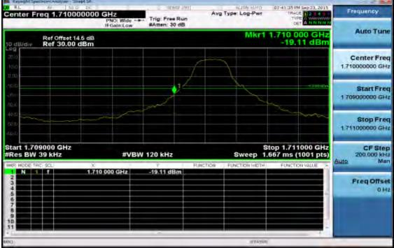
Band edge emission at antenna terminals –3MHz BW LTE-Band 4 (QPSK RB Number: 1 Offset: 14) Channel Highest
