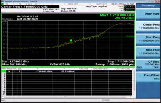
Band edge emission at antenna terminals –15MHz BW LTE-Band 4 (QPSK RB Number: 1 Offset: 74) Channel Highest
