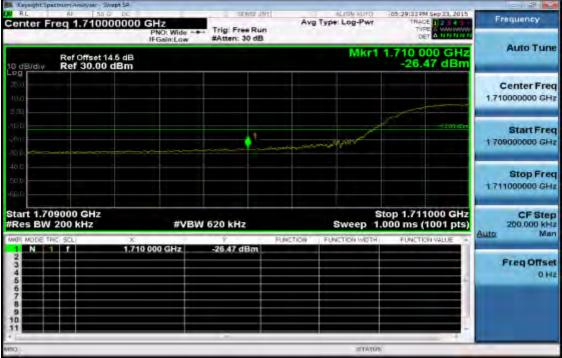
Band edge emission at antenna terminals –15MHz BW LTE-Band 4 (QPSK RB Number: 75 Offset: 0) Channel Highest
