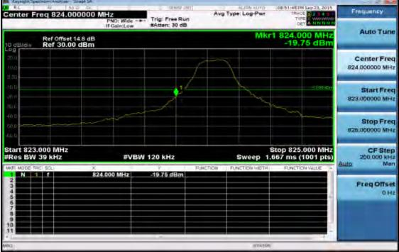
Band edge emission at antenna terminals –3MHz BW LTE-Band 5 (QPSK RB Number: 1 Offset: 14) Channel Highest
