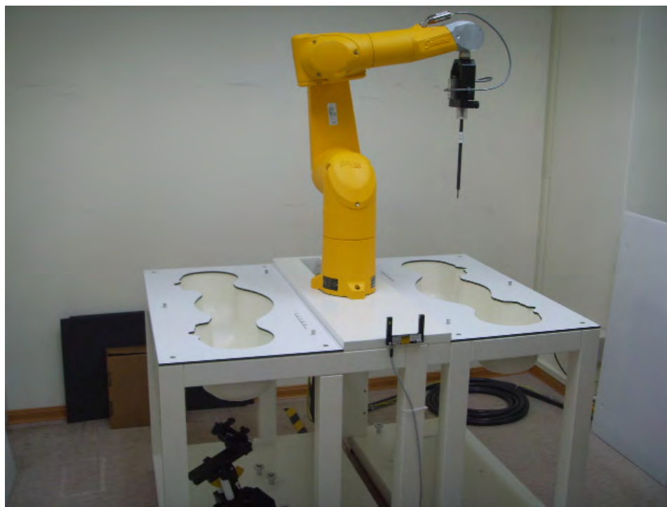
Fig.1 Photograph of the SAR measurement system
