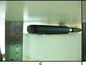
The right edge of the EUT face to the phantom with 5mm-separation distance.
