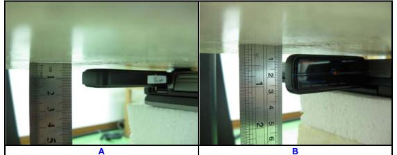
The bottom of the EUT face to the phantom with 5mm-separation distance.
