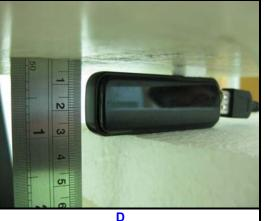
The front of the EUT face to the phantom with 5mm-separation distance.
