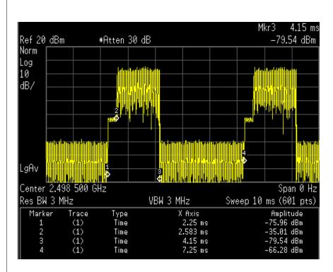
16QAM 3/4 Mkr4 6.65 ms Ref 20 dBm #Atten 30 dB -98.18 dBm Norm Log 10 dB/ ut M.M. Ind ر ک LgAv ł Center 2.498 500 GHz Span 0 Hz Res BW 3 MHz VBW 3 MHz Sweep 10 ms (601 pts) Amplitude -83.27 dBm -40.61 dBm X Axis 1.65 ms 2.017 ms 3.583 ms Marker Trace Туре (1)Time 1 (1)2 Time 3 (1)Time -81.78 dBm -98.18 dBm 4 (1)Time 6.65 ms Duty cycle calculated formula = ( Mark 3 - Mark 2 ) / ( Mark 4 - Mark 1 ) \*100 % Duty cycle (%) Modulation
