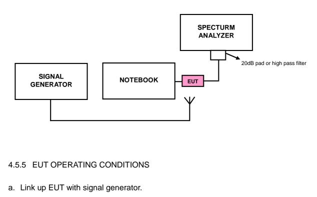
b. The signal generator controlled EUT to export rated output power under transmission mode and specific channel frequency.
