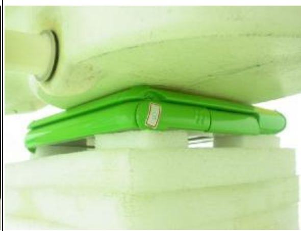
B: The bottom of the EUT face to the phantom with 0mm-separation distance.
