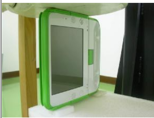
A: The edge of the EUT face to the phantom with 0mm-separation distance.
