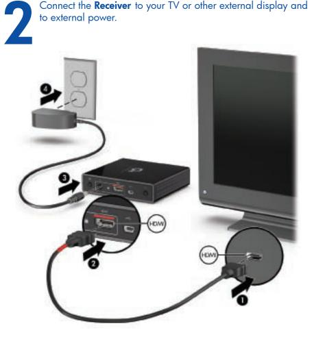
If you connected to a TV, press the input source button on the TV to select the HDMI input. When the components are connected correctly and the correct source is selected, the image on the computer display will be shown on the TV.
