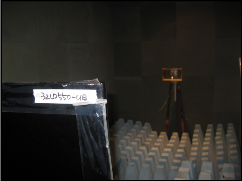
Radiated test setup
