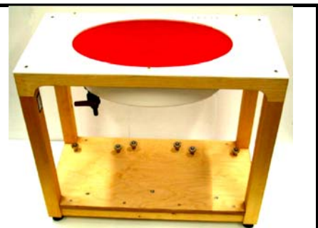
Fig 5.7 Photo of ELI4 Phantom
