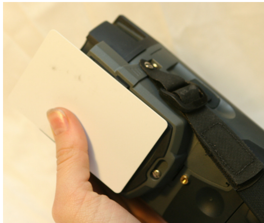
Figure 7 - Handling a contactless smart card properly in order to read it flawlessly
