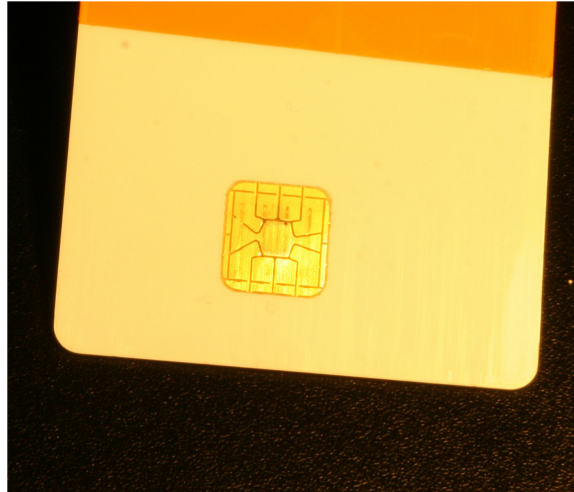
Figure 4 - Zoomed view of the contacts of a smart card
