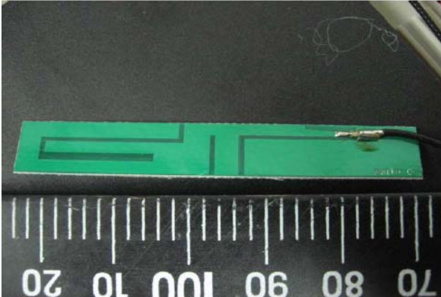
Front View of Mobile Antenna and Dimension
