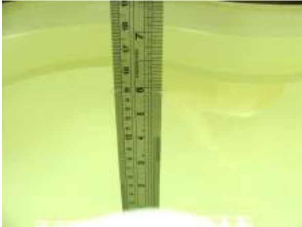
Fig 6.1 Photo of Liquid Height for Head SAR
