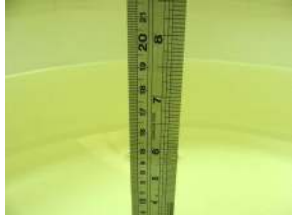
Fig 6.2 Photo of Liquid Height for Body SAR
