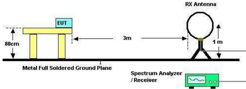
For radiated emissions from 30MHz to 1GHz
