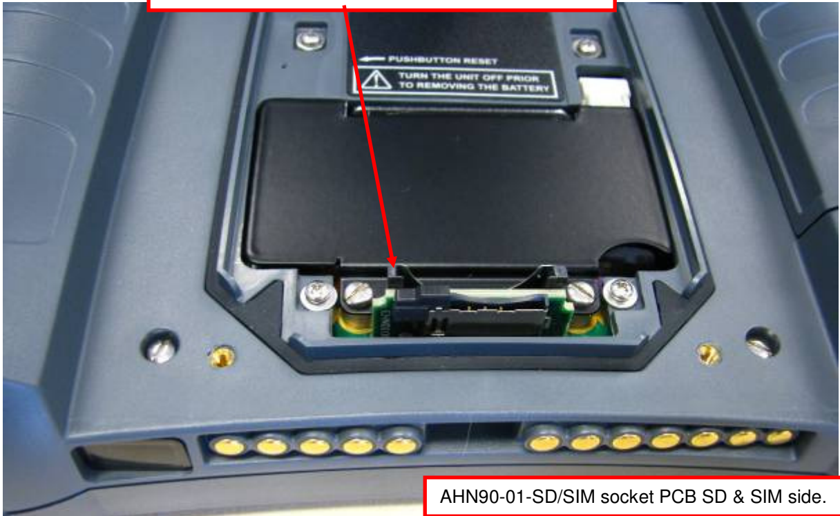
AHN90-01-SD/SIM socket PCB location in unit.
