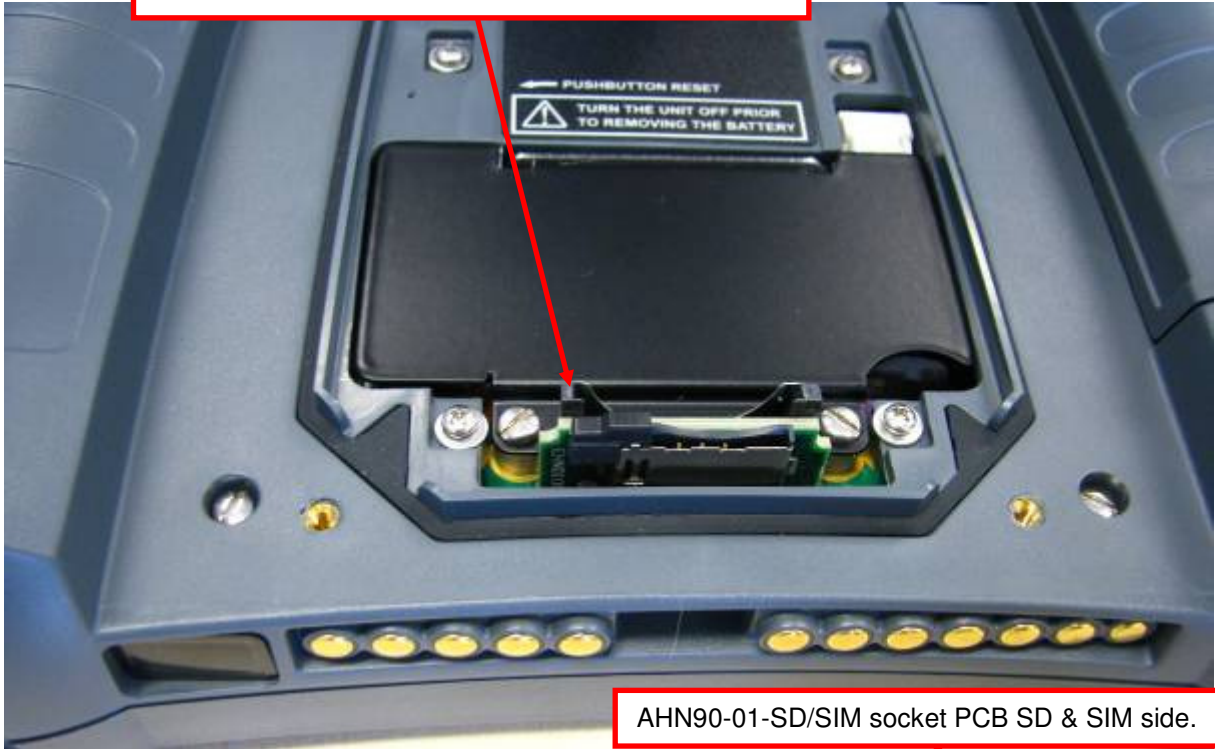
AHN90-01-SD/SIM socket PCB location in unit.
