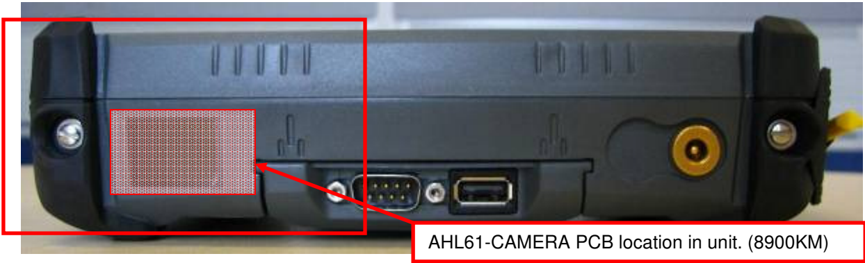
AHL61- CAMERA Top & Bottom PCB. (8900KM)
