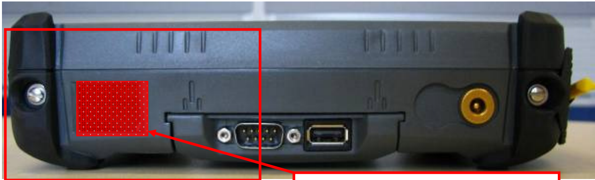
AGE31-RJ45 connector location in unit.
