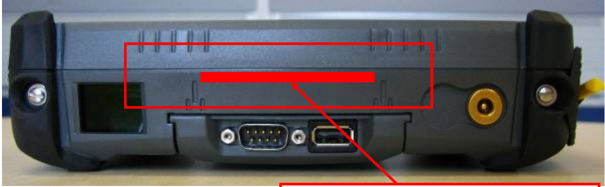
AHN62-GPS interconnect PCB location in unit.
