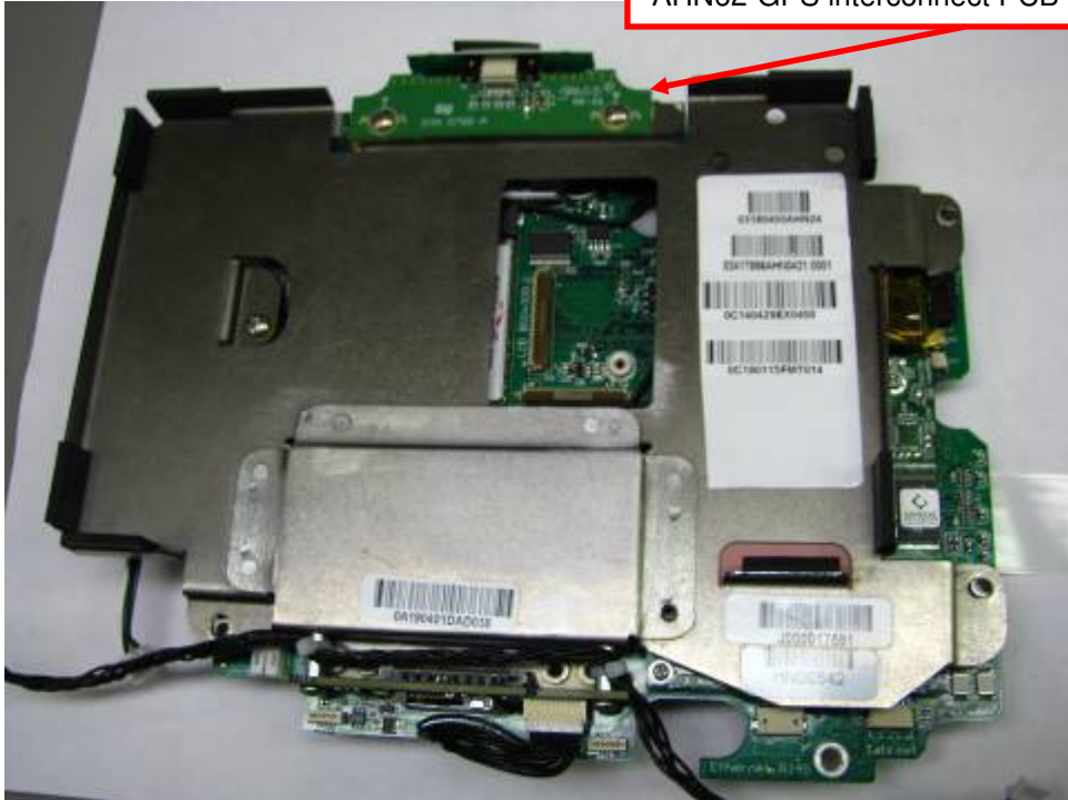
AHN62-GPS interconnect PCB location in unit.
