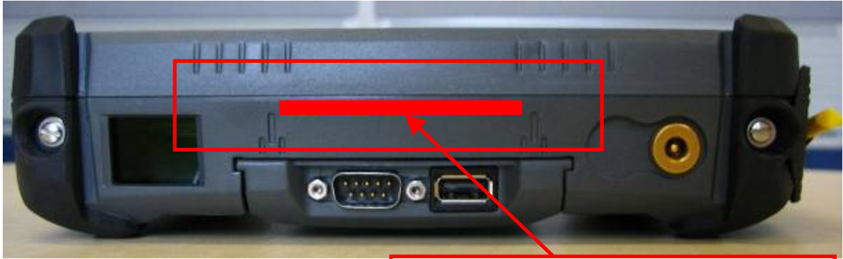
AHN62-GPS interconnect PCB location in unit.
