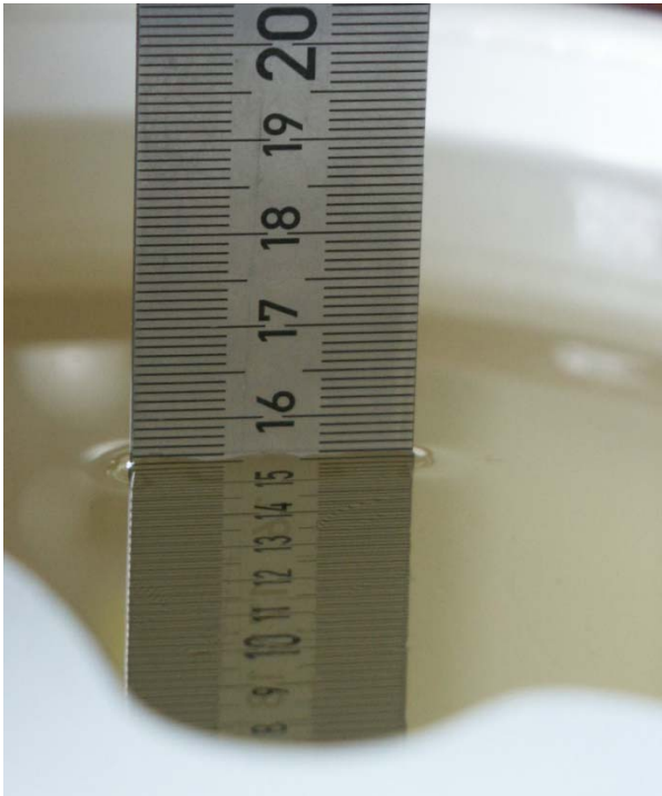
Fig. 29: Liquid depth for GPRS 850 body measurements.
