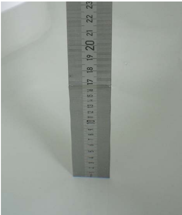
Fig. 31: Liquid depth for IEEE 802.11 body measurements.
