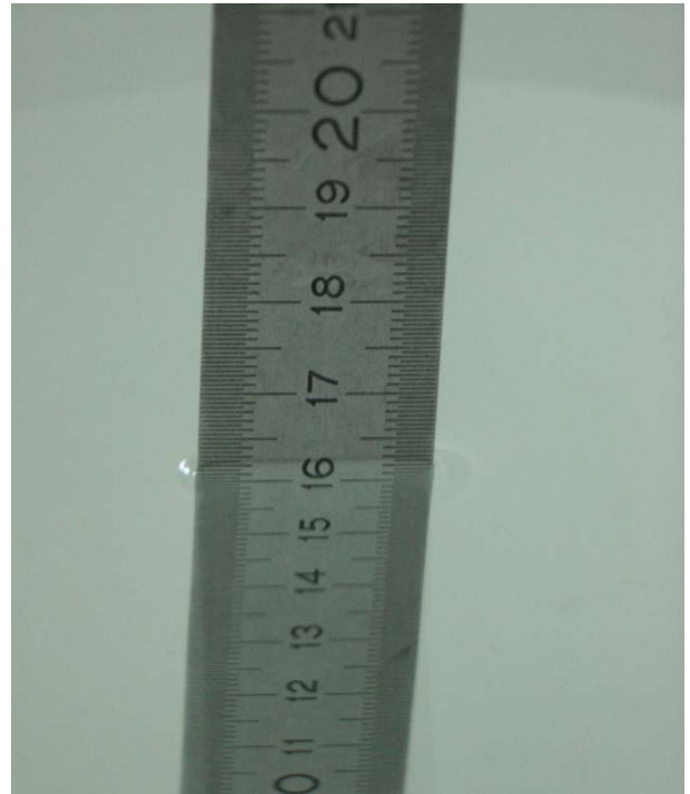
Fig. 30: Liquid depth for GPRS 1900 body measurements.
