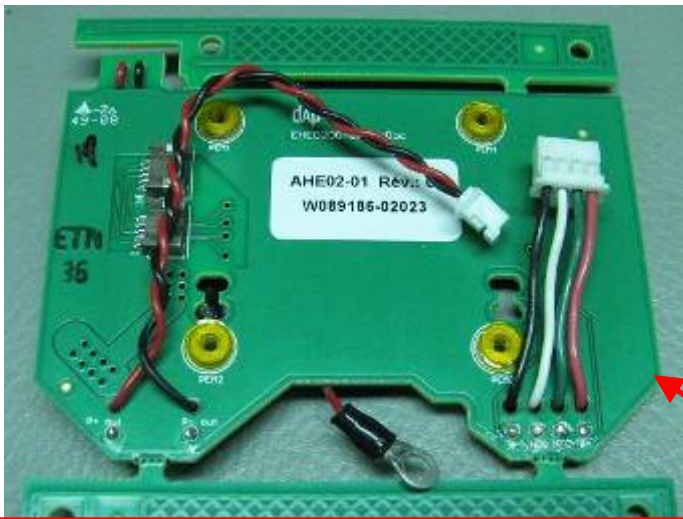
EHE0200-BATTERY interface PCB-Top side with crackers to be removed before installation in unit.
