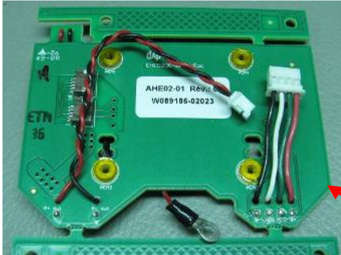
EHE0200-BATTERY interface PCB-Top side with crackers to be removed before installation in unit.
