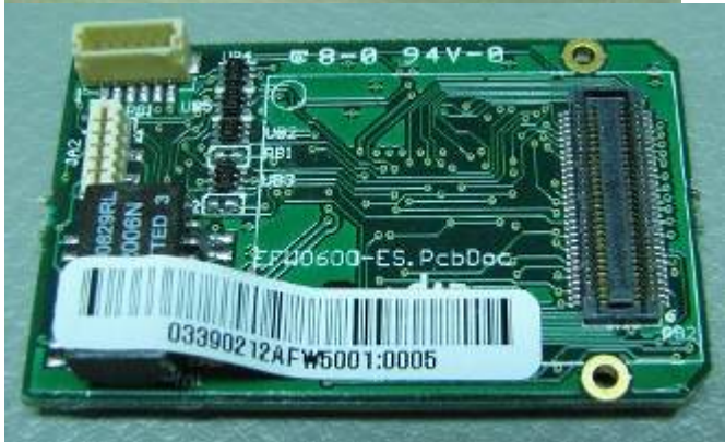
EFW0600-WIFI/BT/ETHERNET PCB TOP
