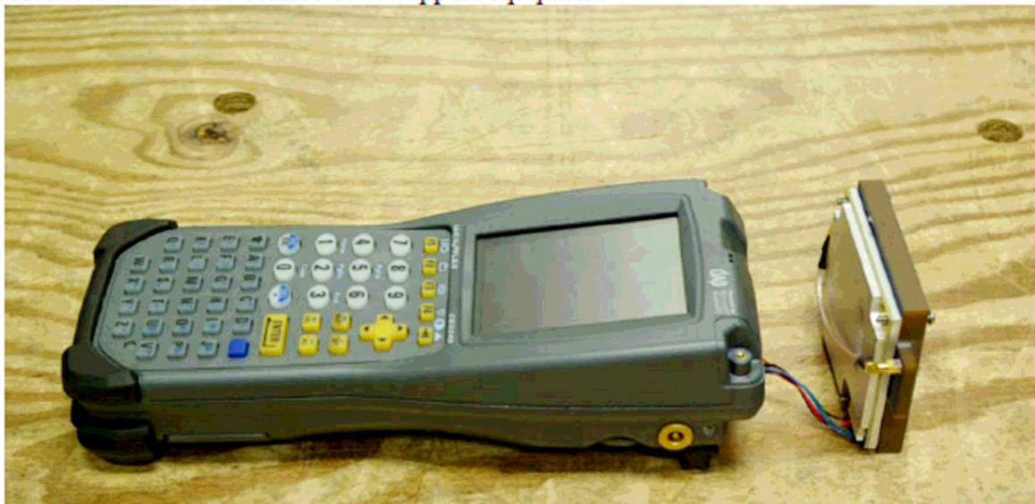
Transceiver module connected to support equipment
