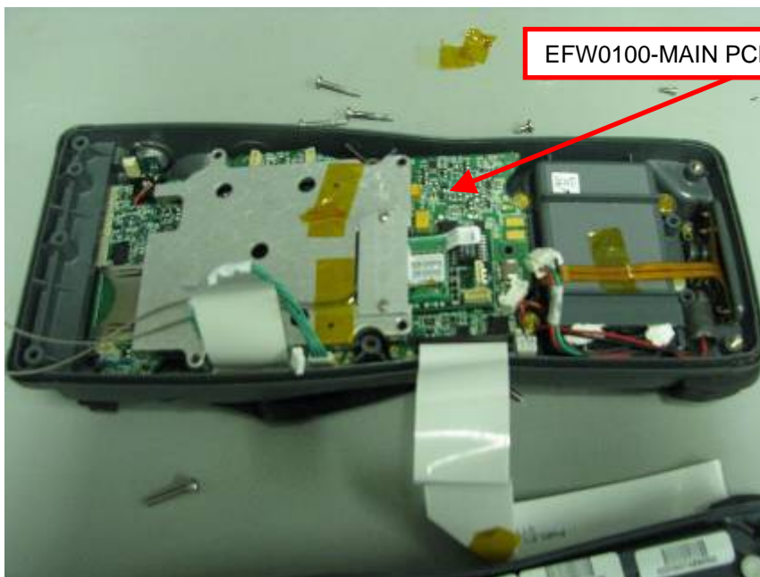
Bottom shell for standard battery configuration inside view
