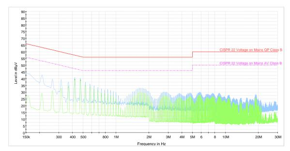
Conducted Emission in charging mode on Phase Line
