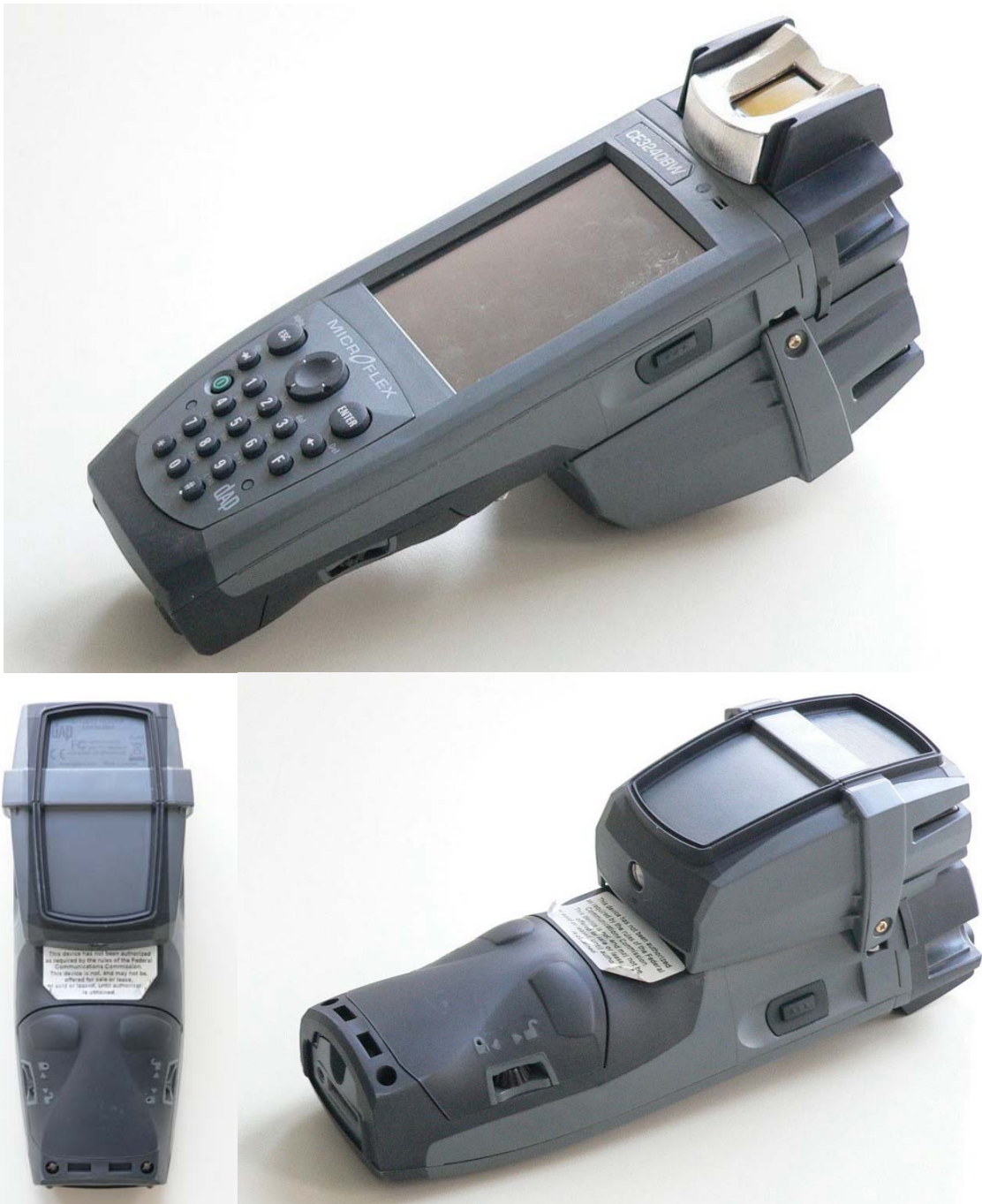
Fig. 17: Pictures of the device 3000B4 with attached smart card reader.
