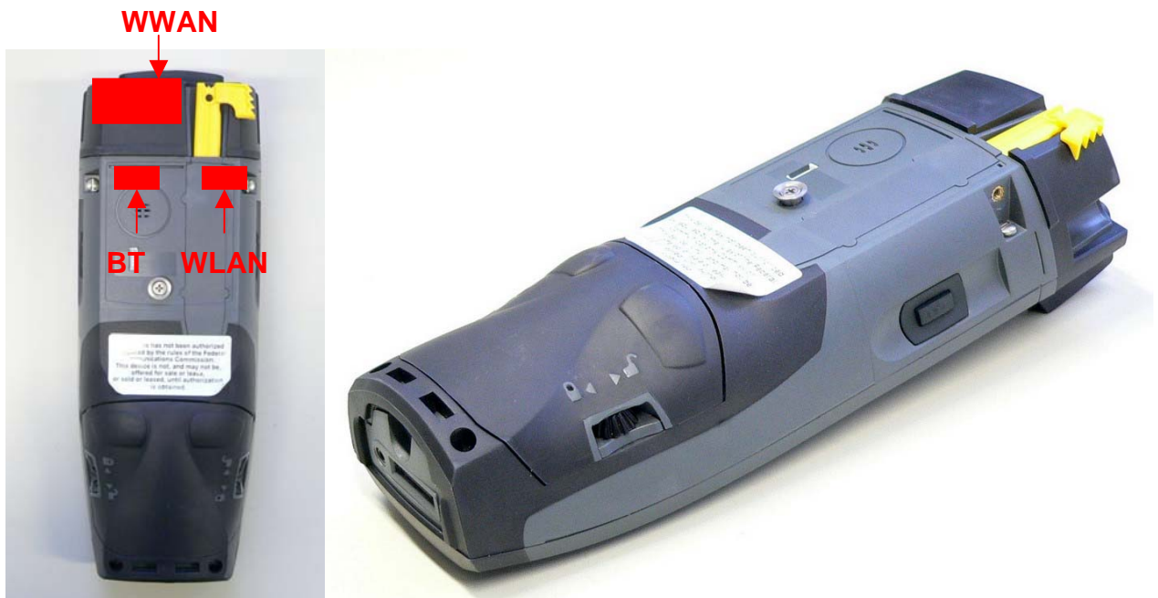
Fig. 16: Back view of the device 3000B4 without the smart card reader and Antenna positions
