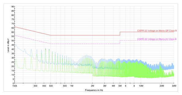
Conducted Emissions in charging mode on Neutral Line CISPR 22 Voltage on Mains QP Class B.LimitLine CISPR 22 Voltage on Mains AV Class B.LimitLine Preview Peak Result Preview Average Result \* Final Average Result
