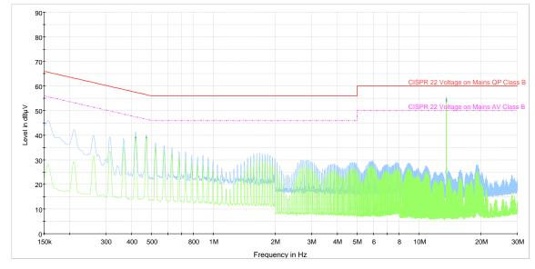
Conducted Emissions in charging mode on Phase Line Cred Emission's in charging mode on Phase Line CISPR 22 Voltage on Mains AV Class B.LimitLine CISPR 22 Voltage on Mains AV Class B.LimitLine Preview Pak Result Preview Average Result Final Average Result Final Average Result
