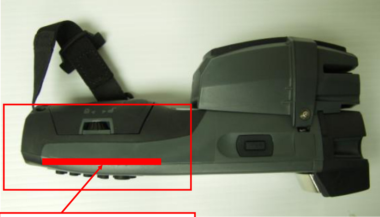
EGF0200-KEYBOARD PCB-location in unit.
