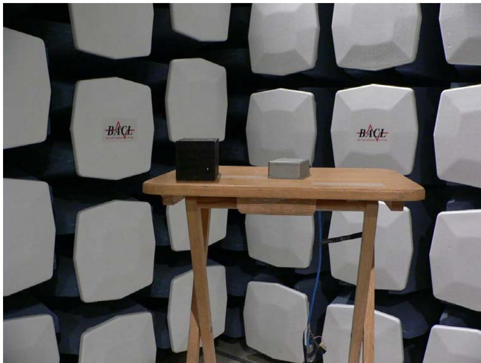
**PT5-UHF: Radiated Emission - Rear View**
